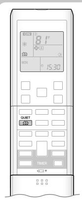
OUTDOOR UNIT QUIET operation lowers the noise level of the outdoor unit by changing the frequency and fan speed on the outdoor unit. This function is convenient during the night.
