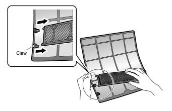
**2.** Clean or replace the titanium apatite photocatalytic airpurifying filter.
