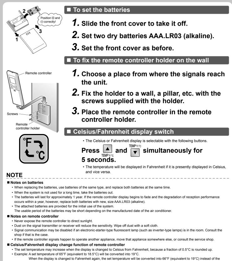
original set temperature (65°F) but a set temperature of 66°F (equivalent to 19°C) will be converted into 19°C with no temperature change. • A reception sound will go off for the transmission of set temperature to the indoor unit at the time of setting the Celsius/Fahrenheit display change function.
