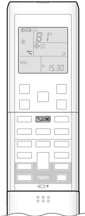
ECONO operation is a function which enables efficient operation by limiting the maximum power consumption value.
