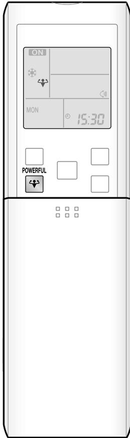
POWERFUL operation quickly maximizes the cooling (heating) effect in any operation mode. You can get the maximum capacity.
