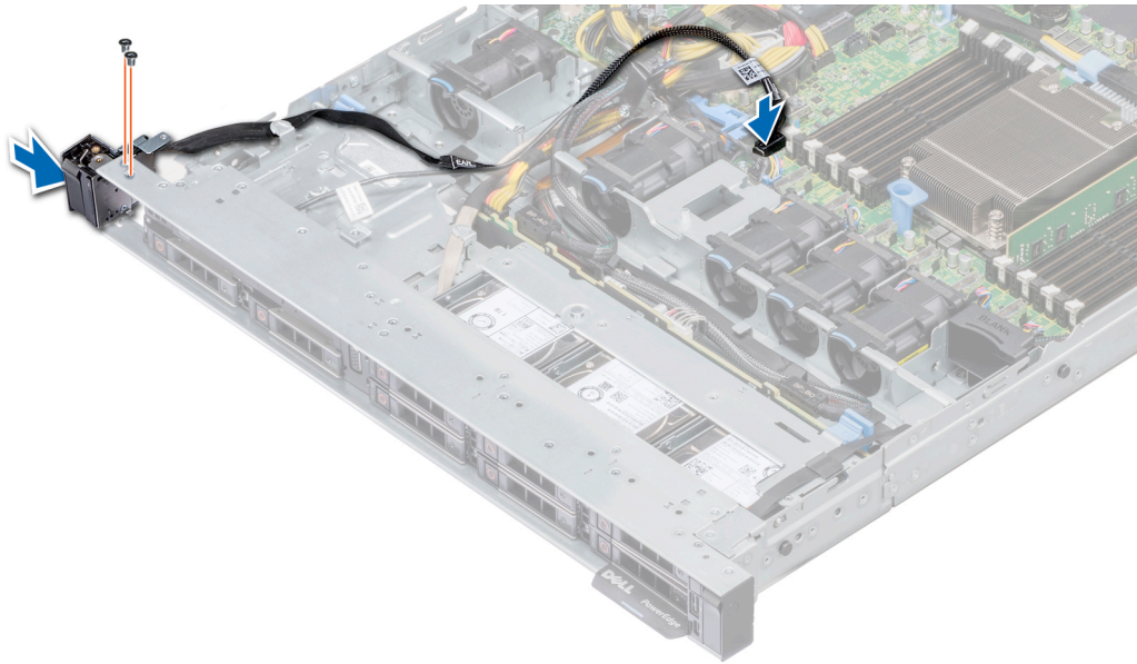
Figure 92. Installing the left control panel
