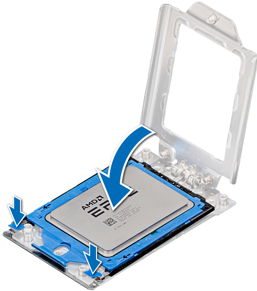
Figure 49. Closing the processor socket frame
