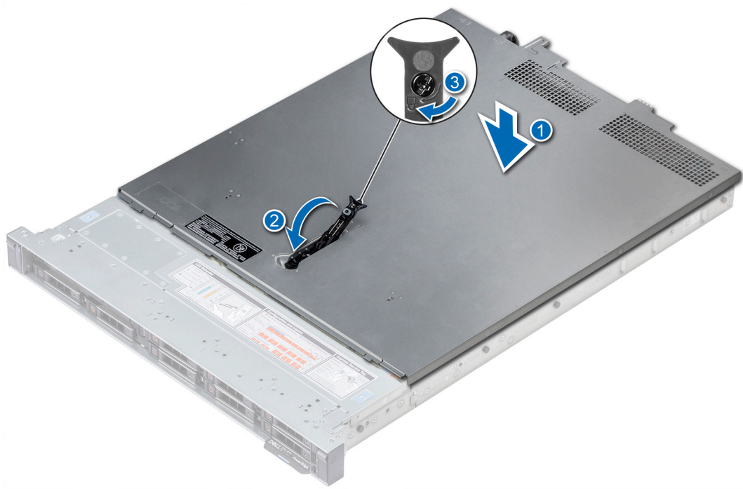
Figure 25. Installing system cover
