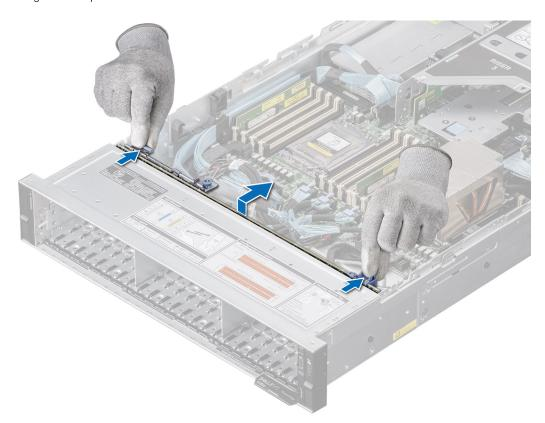
Figure 52. Removing the drive backplane
