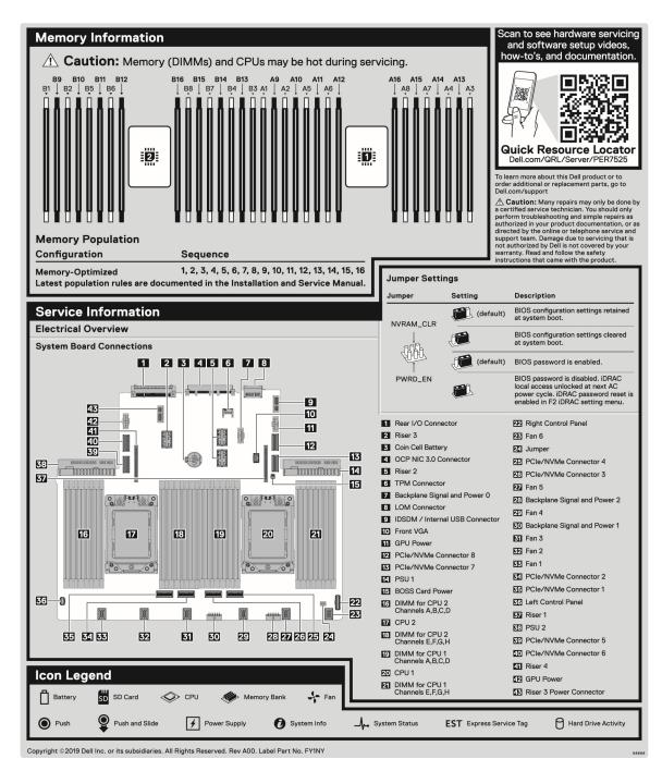
Figure 15. Memory information and system board connectors
