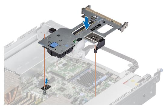
Figure 94. Installing the expansion card riser (Riser 2)
