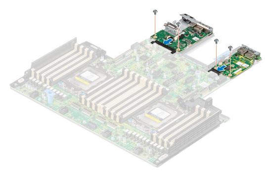
Figure 152. Installing the RIO card
