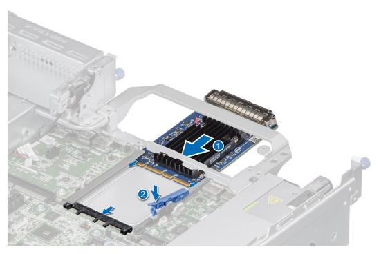
Figure 143. Installing the OCP card
