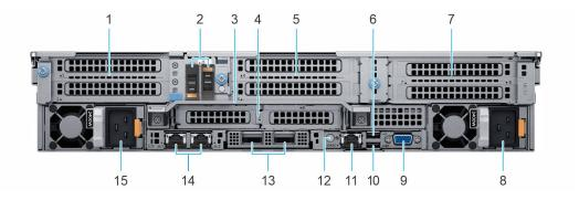
Figure 9. Rear view of the system
