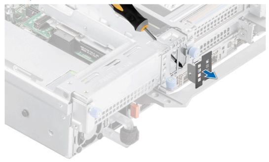
Figure 153. Removing the BOSS blank
