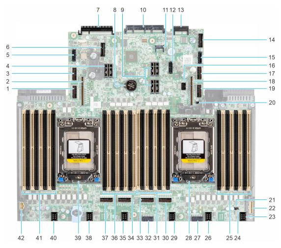
Figure 158. System board jumpers and connectors
