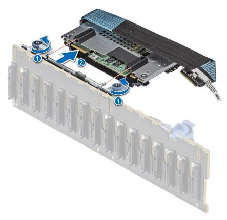
Figure 72. Removing the rear mounting front PERC module
