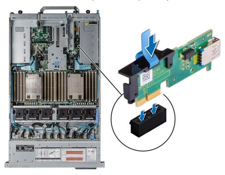
Figure 137. Installing the internal USB card
