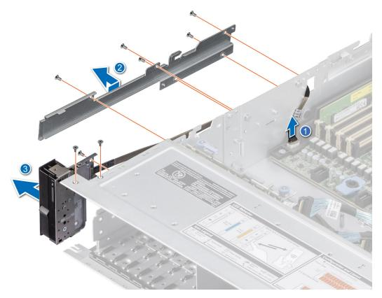
Figure 26. Removing the left control panel
