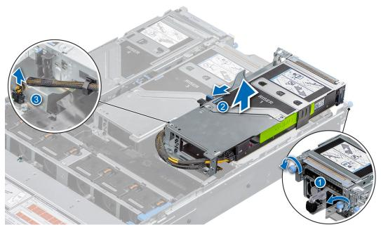
Figure 102. Removing the expansion card riser (Riser 1A)
