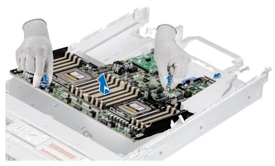
Figure 147. Removing the system board
