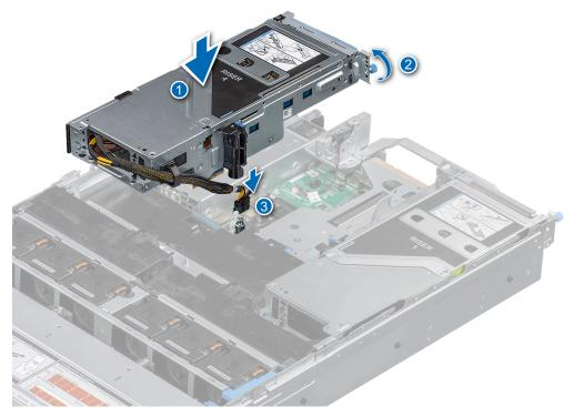
Figure 107. Installing the expansion card riser (Riser 4A)
