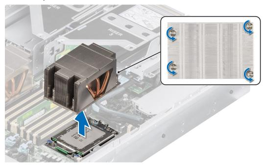
Figure 77. Removing a heat sink
