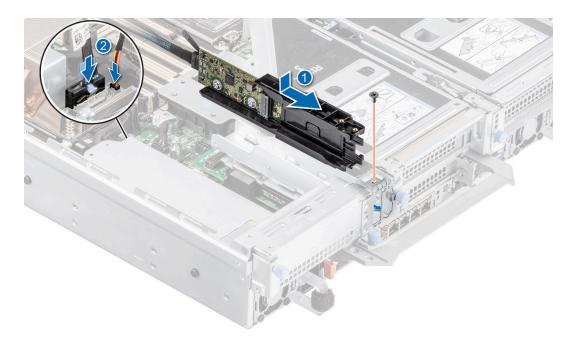
Figure 131. Installing the BOSS S2 controller card module
