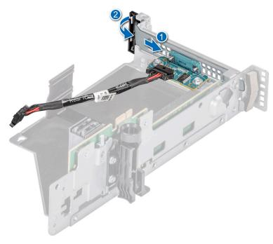
Figure 116. Installing the Serial COM port
