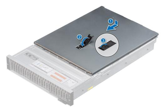
Figure 21. Installing the system cover
