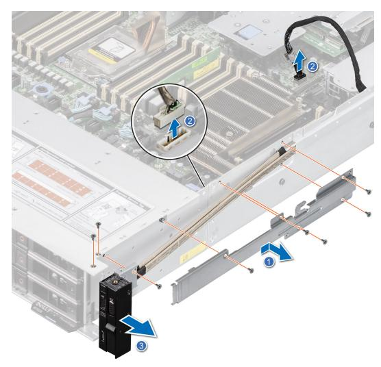
Figure 24. Removing the right control panel
