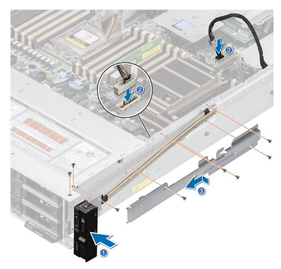
Figure 25. Installing the right control panel
