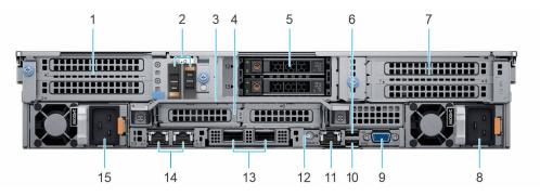
Figure 10. Rear view of the system with 2 x 2.5-inch rear drive module
