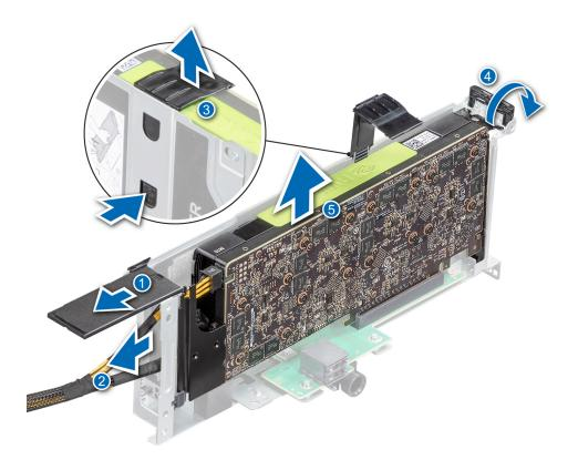
Figure 109. Removing GPU 3 and 4
