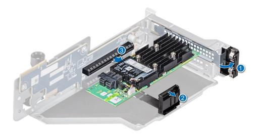
Figure 97. Removing expansion card from the expansion card riser
