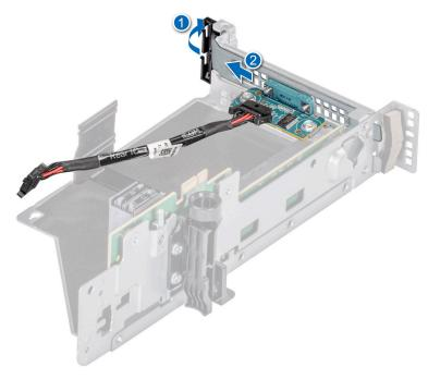
Figure 114. Removing the Serial COM port
