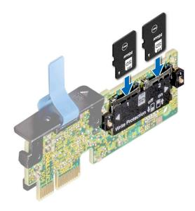
Figure 121. Installing the MicroSD card
