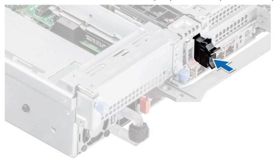
Figure 125. Installing the BOSS card filler
