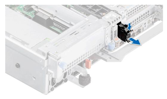
Figure 124. Removing the BOSS card filler
