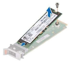
Figure 127. Removing the M.2 SSD
