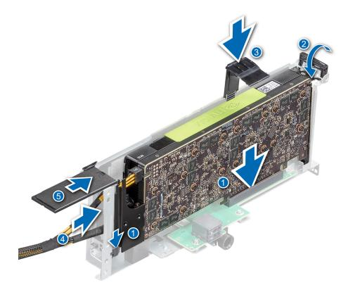
Figure 113. Installing GPU on Riser 3 and Riser 4
