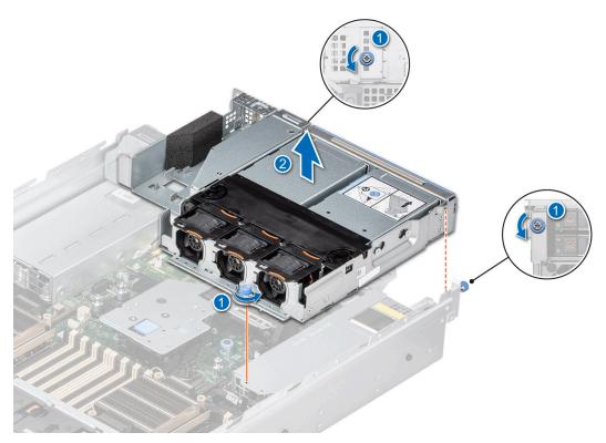
Figure 66. Removing the 4 x 2.5-inch rear drive module
