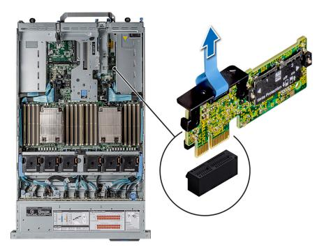
Figure 118. Removing the IDSDM module
