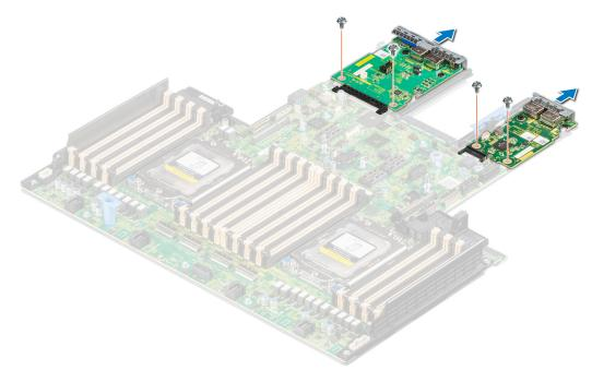
Figure 151. Removing the RIO card
