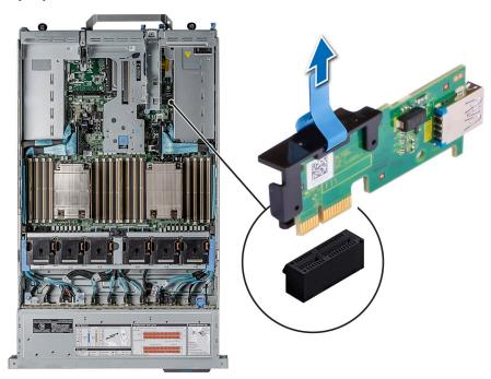
Figure 136. Removing the internal USB card
