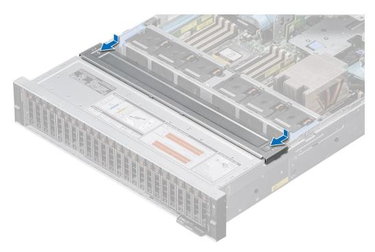
Figure 23. Installing the drive backplane cover
