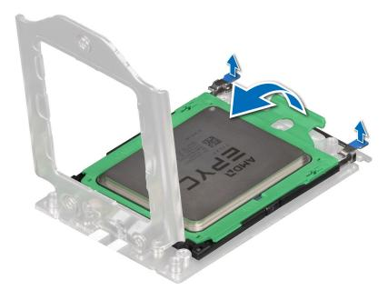
Figure 80. Lifting the rail frame
