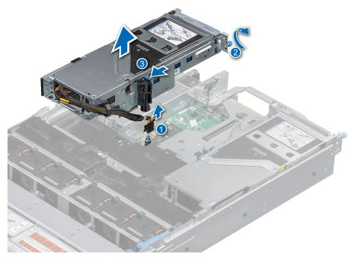
Figure 104. Removing the expansion card riser (Riser 4A)
