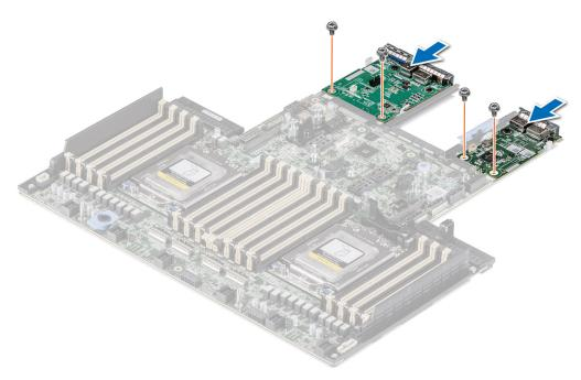
Figure 150. Installing the LOM card and rear I/O board
