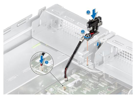
Figure 139. Installing the intrusion switch module
