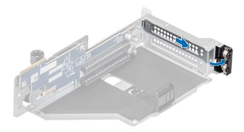
Figure 99. Removing the filler bracket
