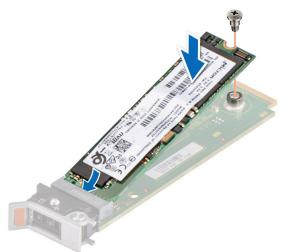
Figure 132. Installing the M.2 SSD
