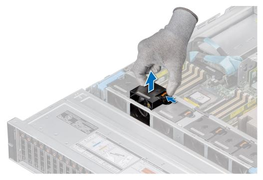
Figure 36. Removing a cooling fan
