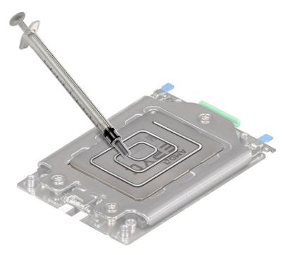
Figure 85. Applying thermal grease
