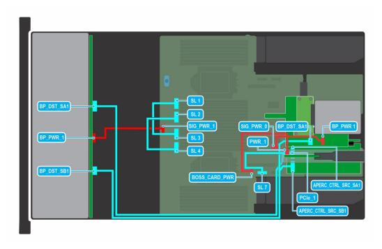
Figure 56.  $12 \times 3.5$ -inch with rear hard drives
