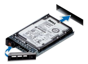
Figure 43. Installing a drive carrier
