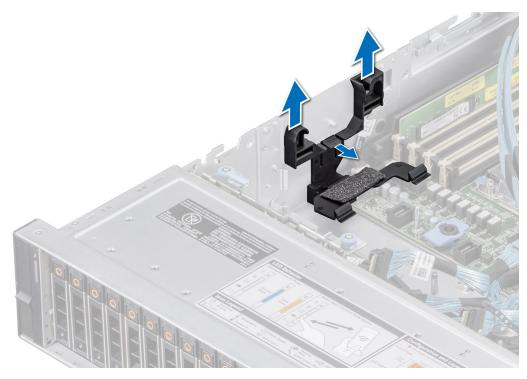
Figure 38. Removing the side wall bracket
