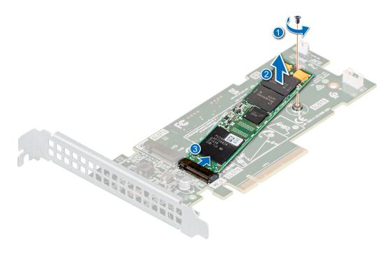
Figure 122. Removing the M.2 SSD module
