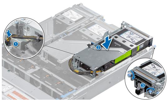
Figure 105. Installing the expansion card riser (Riser 1A)
