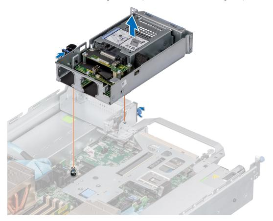
Figure 68. Removing the rear drive cage
