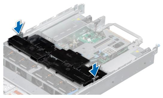
Figure 31. Installing the GPU air shroud
