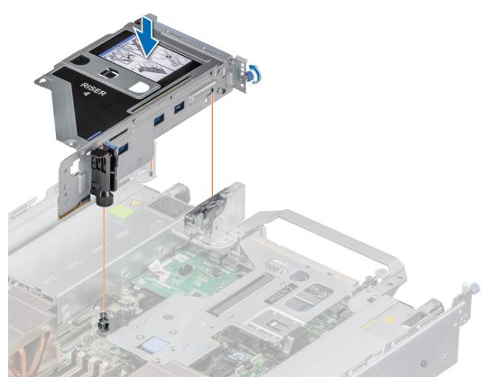
Figure 96. Installing the expansion card riser (Riser 4)
