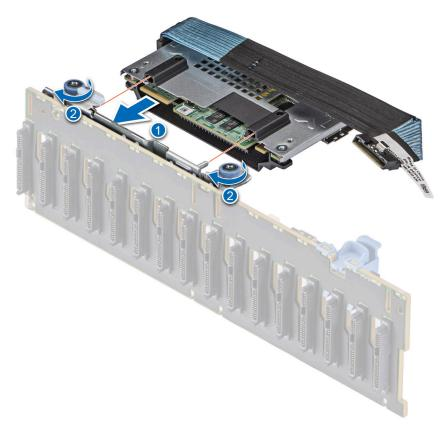
Figure 73. Installing the rear mounting front PERC module
