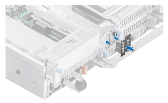
Figure 154. Installing the BOSS blank
