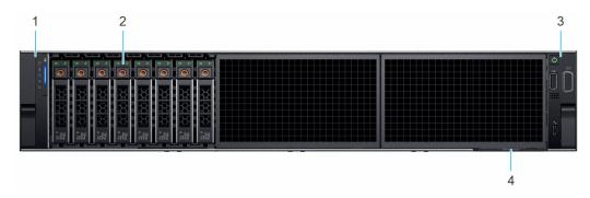
Figure 3. Front view of the  $8 \times 2.5$ -inch drive system
