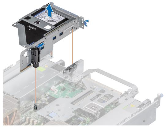
Figure 92. Removing the expansion card riser (Riser 4)
