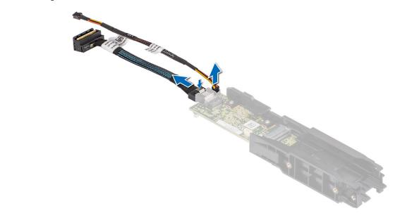
Figure 101. Removing the BOSS power cable and BOSS signal cable from the BOSS S2 controller card module
