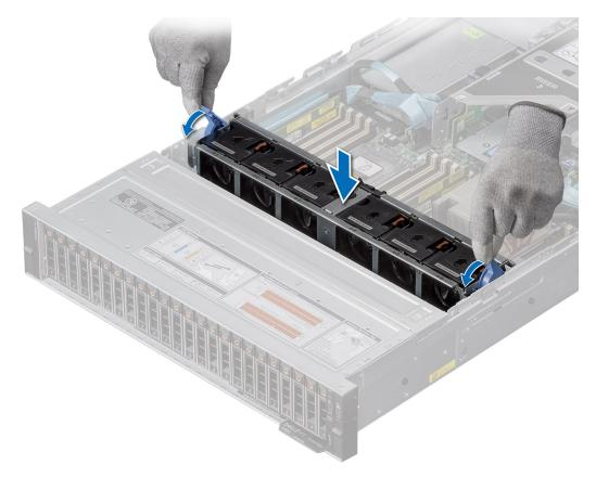
Figure 35. Installing the cooling fan cage assembly
