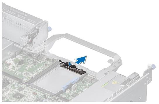
Figure 142. Removal of filler bracket
