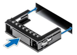
Figure 41. Installing a drive blank
