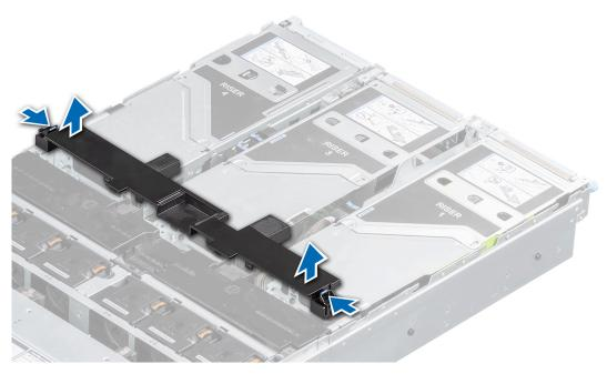
Figure 32. Removing the GPU air shroud top cover
