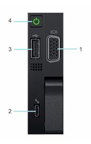
Figure 8. Right control panel view
