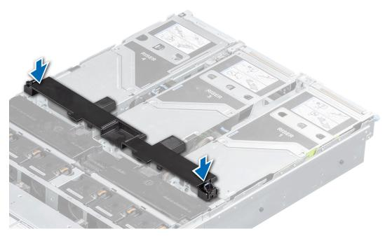
Figure 33. Installing the GPU air shroud top cover
