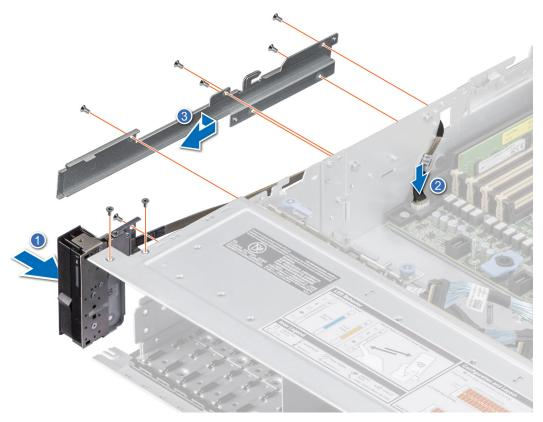
Figure 27. Installing the left control panel
