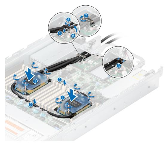
Figure 87. Installing the liquid cooling heat sink
