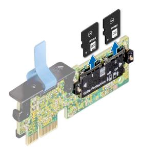
Figure 120. Removing the MicroSD card
