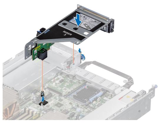
Figure 95. Installing the expansion card riser (Riser 3)
