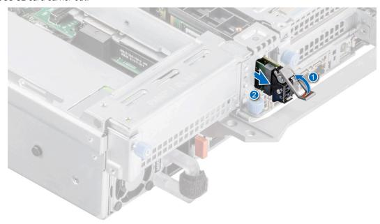
Figure 126. Removing the BOSS S2 card carrier
