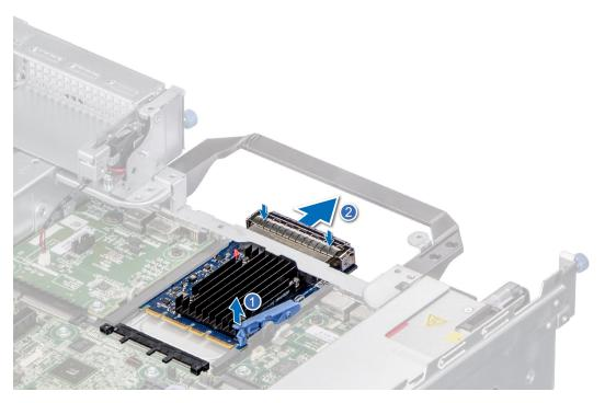
Figure 140. Removing the OCP card
