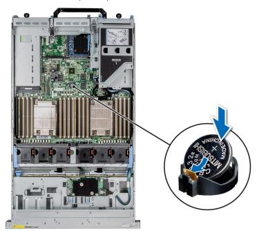
Figure 135. Removing the system battery
