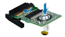
Figure 146. Installing the TPM
