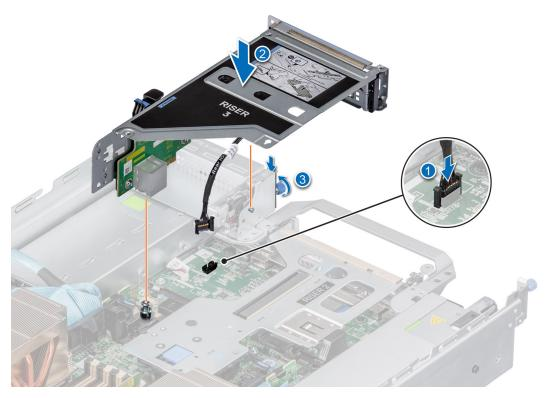
Figure 117. Installing the Serial COM port
