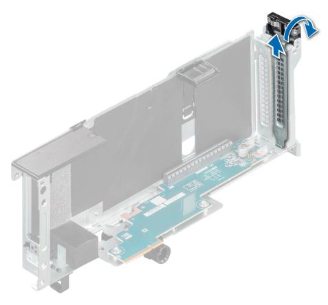
Figure 111. Removing the metal filler bracket
