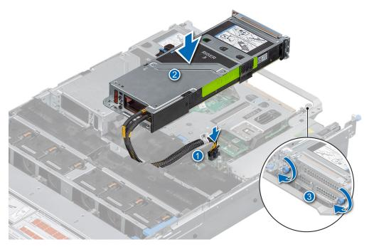
Figure 106. Installing the expansion card riser (Riser 3A)
