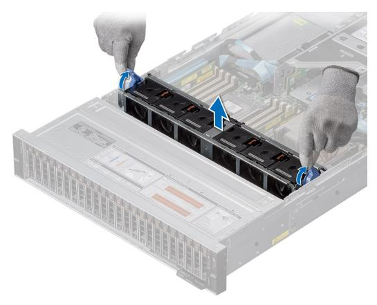
Figure 34. Removing the cooling fan cage assembly
