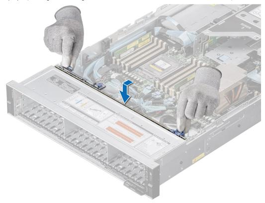
Figure 53. Installing the drive backplane
