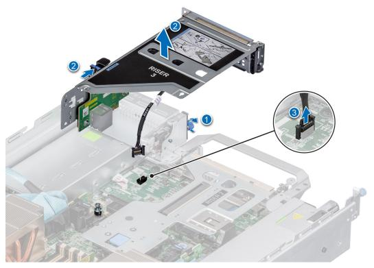
Figure 115. Removing the Serial COM port
