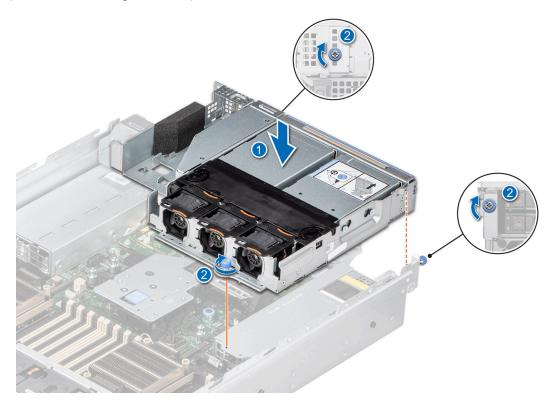
Figure 67. Installing the 4 x 2.5-inch rear drive module
