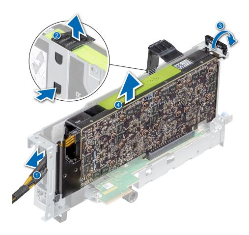
Figure 108. Removing GPU 1
