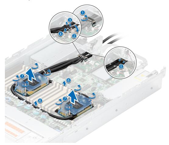
Figure 78. Removing the liquid cooling heat sink modules
