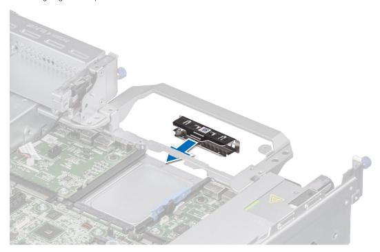
Figure 141. Installation of filler bracket
