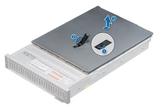
Figure 20. Removing the system cover
