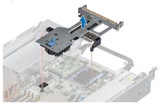
Figure 90. Removing the expansion card riser (Riser 2)
