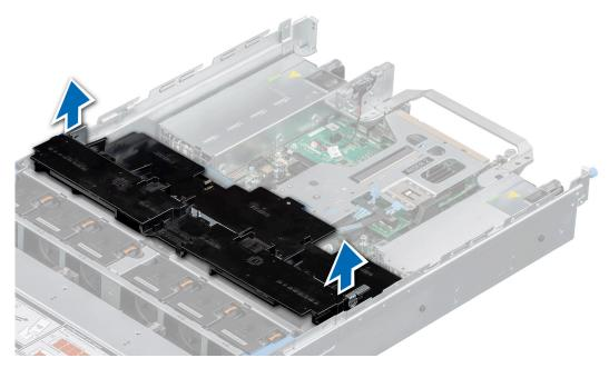
Figure 30. Removing the GPU air shroud
