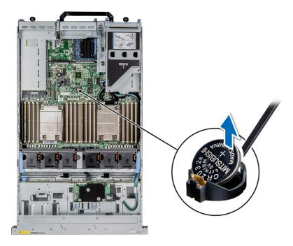
Figure 134. Removing the system battery
