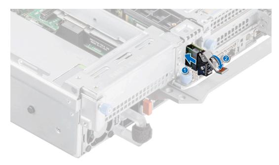
Figure 133. Installing the BOSS S2 card carrier
