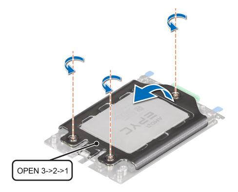
Figure 79. Removing screws on the force plate
