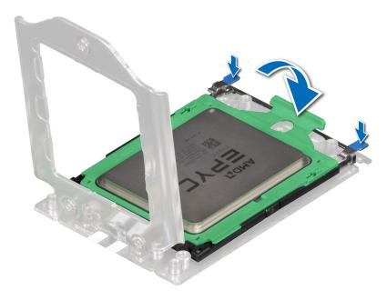
Figure 83. Closing the rail frame
