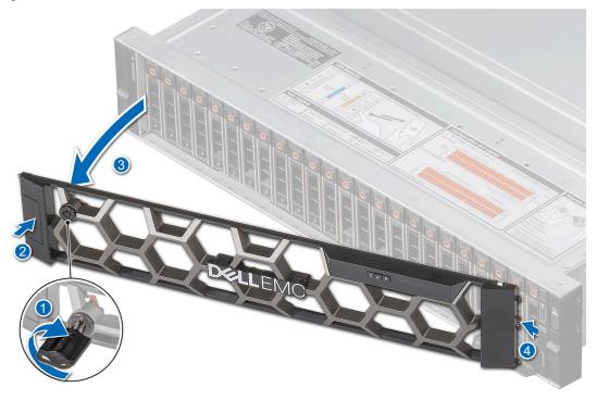
Figure 18. Removing the front bezel
