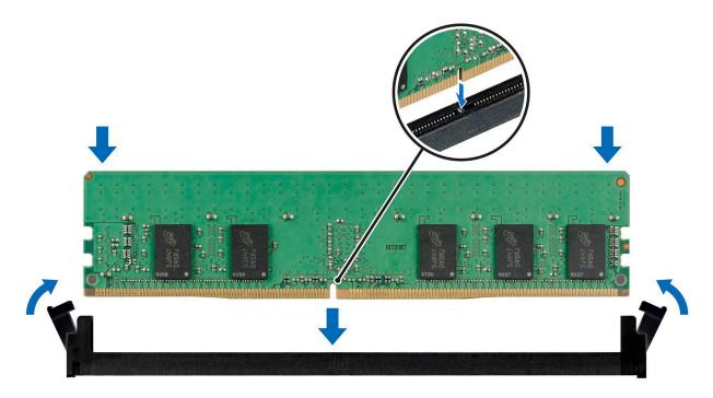
Figure 76. Installing a memory module
