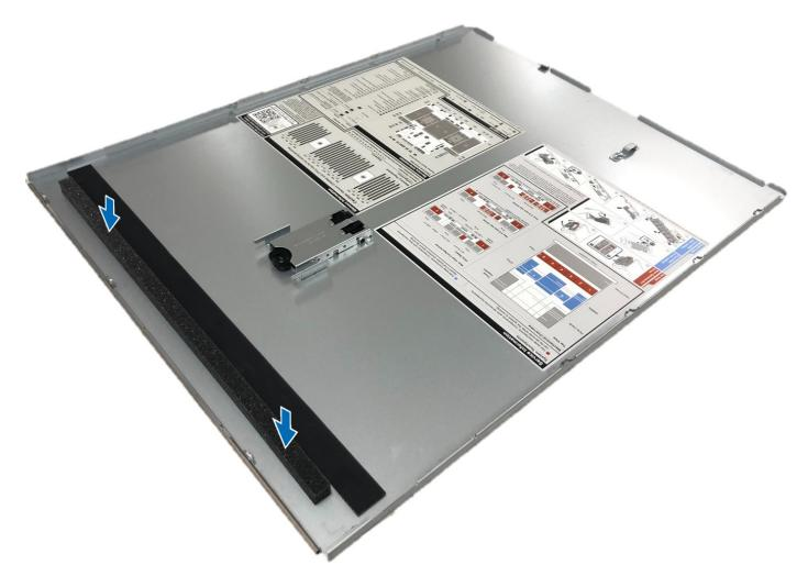
Figure 155. Installing Mylar foam on the system cover
