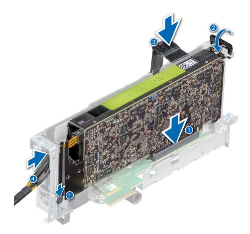
Figure 112. Installing GPU on Riser 1
