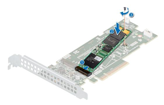
Figure 123. Installing the M.2 SSD module
