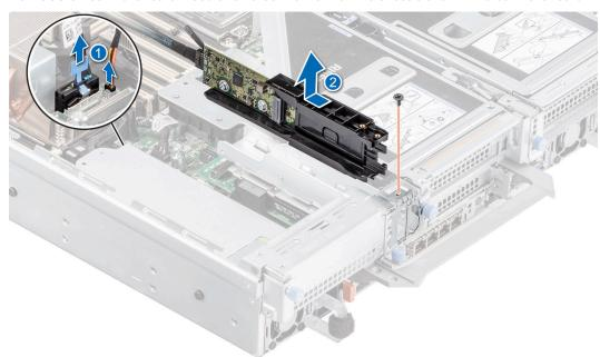
Figure 129. Removing the BOSS S2 controller card module
