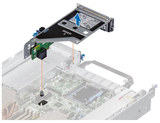
Figure 91. Removing the expansion card riser (Riser 3)
