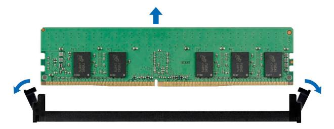
Figure 75. Removing a memory module
