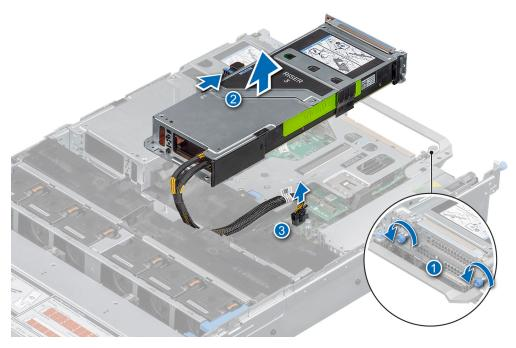
Figure 103. Removing the expansion card riser (Riser 3A)
