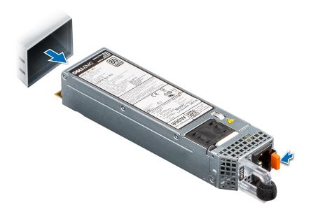
Figure 144. Removing a power supply unit
