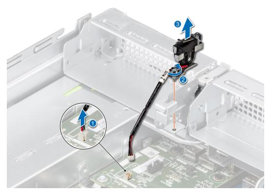
Figure 138. Removing the intrusion switch module
