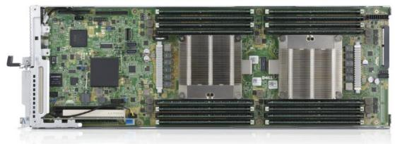
Figure 4. 1U sled — top view
