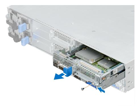
Figure 42. Removing a sled
