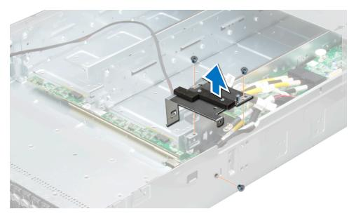
Figure 87. Removing the midplane holder support
