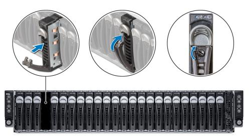
Figure 26. Installing a hard drive carrier
