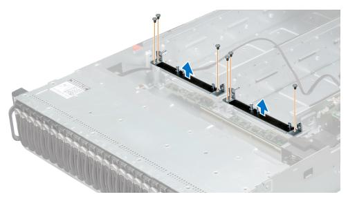
Figure 89. Removing the midplane holder
