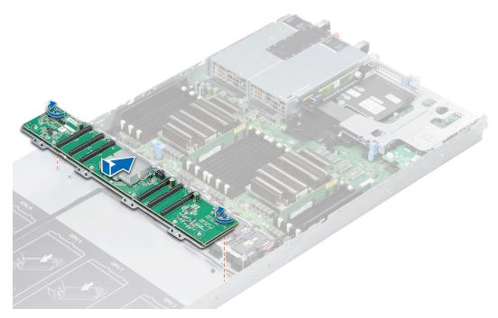
Figure 72. Installing the GPU switch board
