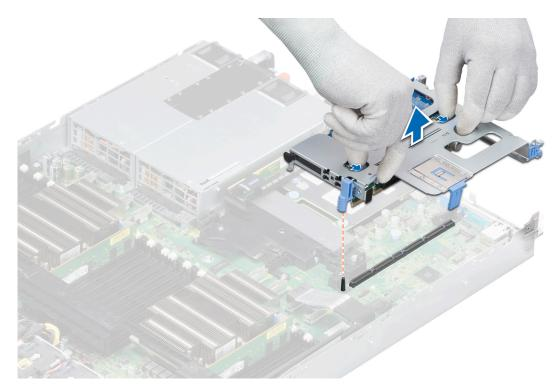
Figure 44. Removing expansion card riser 1
