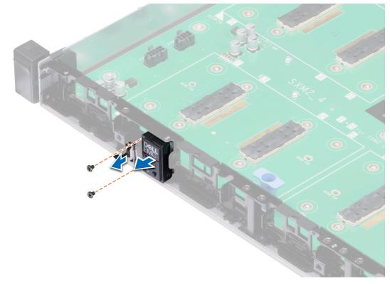
Figure 105. Removing the control panel module
