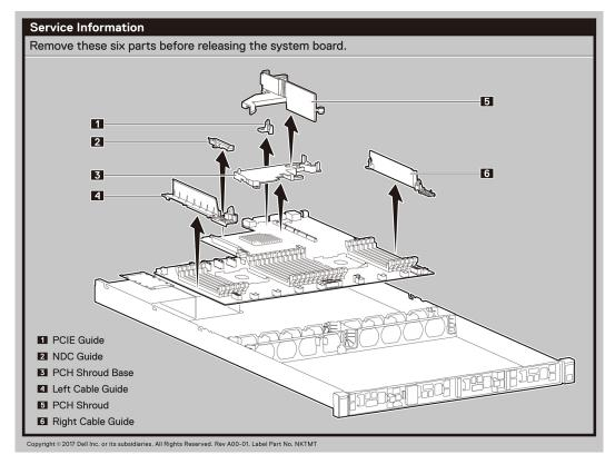
Figure 21. System board removal
