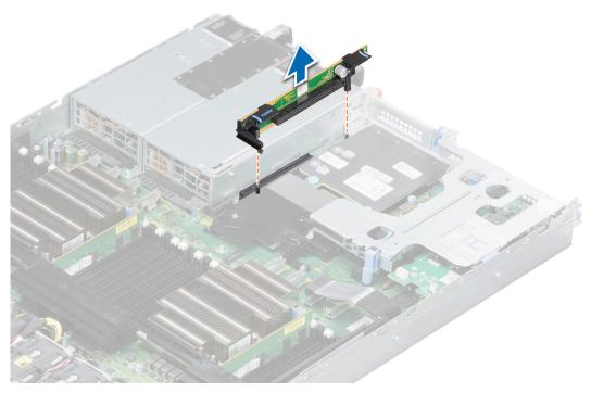
Figure 45. Removing expansion card riser 2
