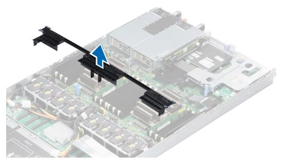
Figure 27. Removing the system air shroud for B, C, G, K and M configurations
