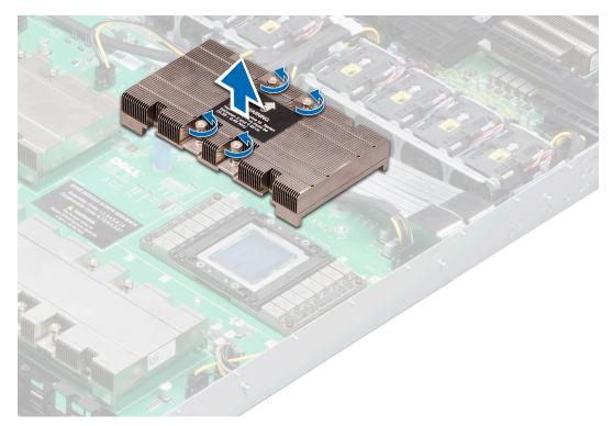
Figure 86. Removing the SXM2-GPU heat sink
