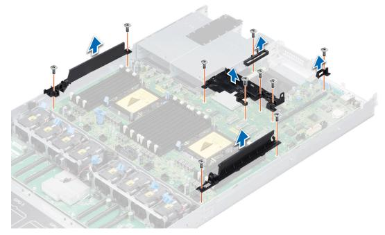
Figure 100. Remove the cable guides, NDC guide, PCIe guide, and PCH shroud base
