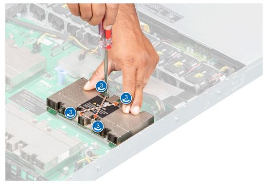
Figure 94. Installing the SXM2-GPU heat sink screws
