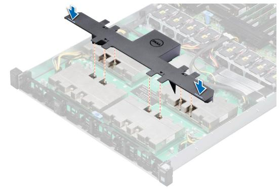
Figure 95. Installing a NVLink air shroud
