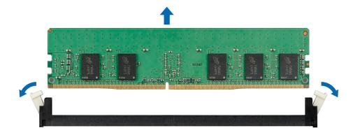
Figure 42. Removing a memory module
