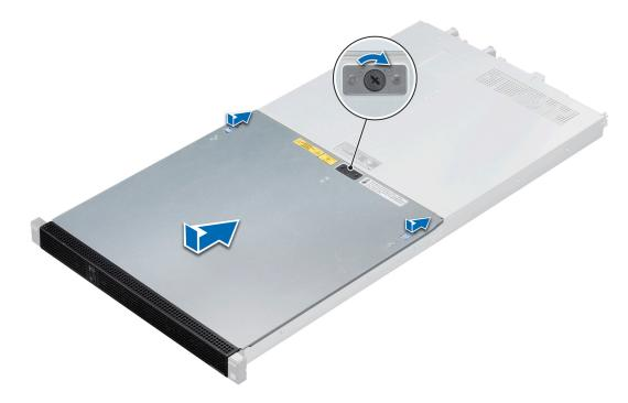
Figure 23. Installing the front system cover
