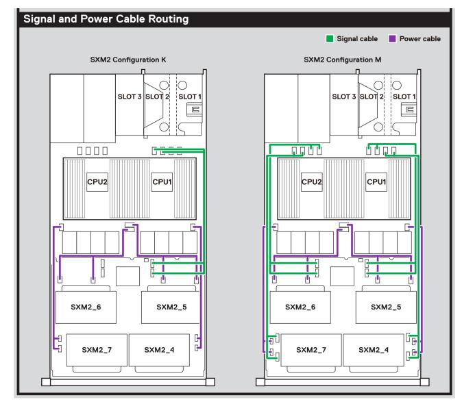
Figure 20. Signal and power cable routing for configurations K and M
