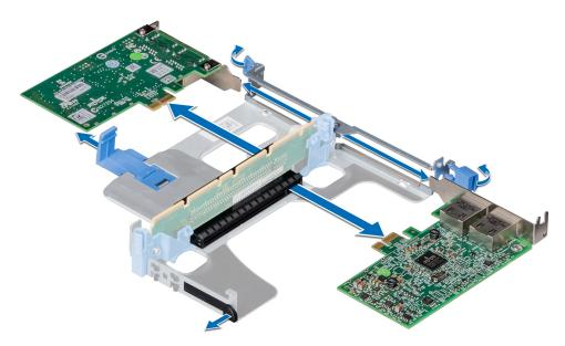
Figure 48. Removing expansion card from riser 1
