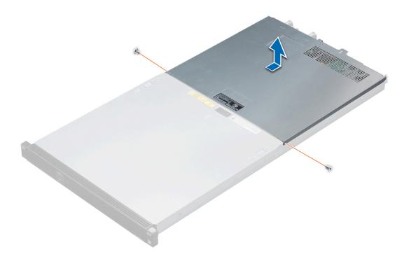
Figure 24. Removing the rear system cover
