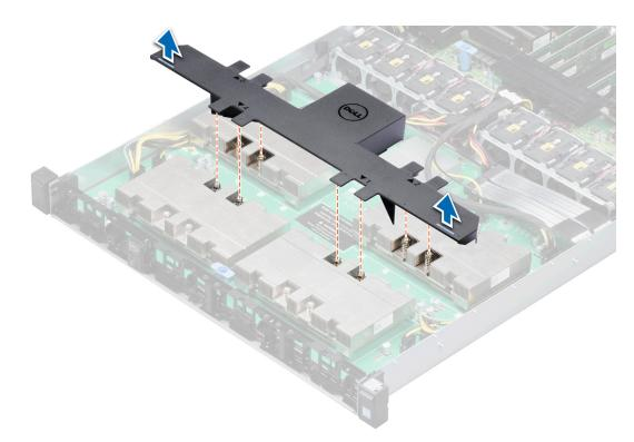
Figure 28. Removing the system air shroud for K and M configurations
