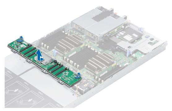
Figure 71. Removing the GPU switch board for configurations B and G
