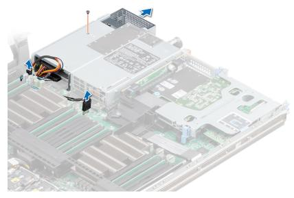
Figure 33. Removing the 2.5-inch drive cage
