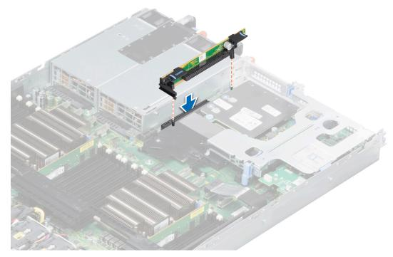
Figure 47. Installing expansion card riser 2
