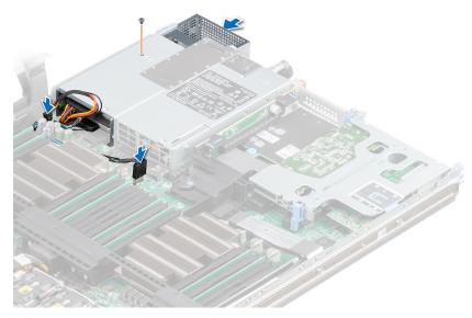
Figure 34. Installing the 2.5-inch drive cage
