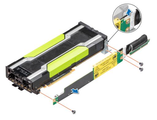
Figure 68. Removing a GPU riser cable board
