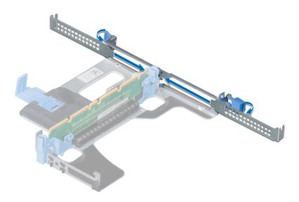
Figure 50. Installing a filler bracket into a riser
