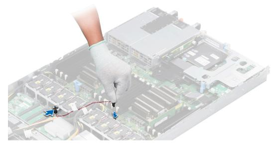
Figure 40. Installing the intrusion switch
