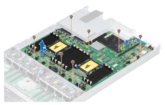
Figure 101. Removing the system board
