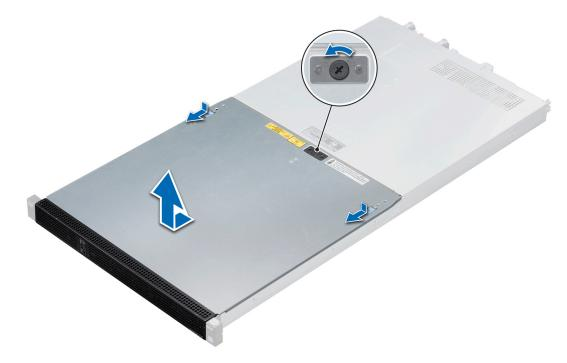
Figure 22. Removing the front system cover
