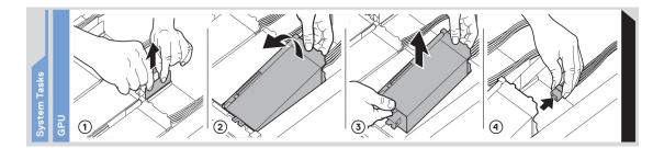
Figure 13. GPU installation
