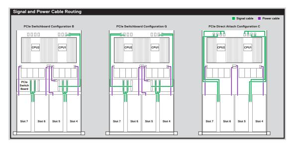
Figure 19. Signal and power cable routing for configurations B, C and G
