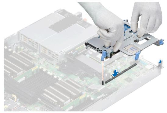
Figure 46. Installing expansion card riser 1
