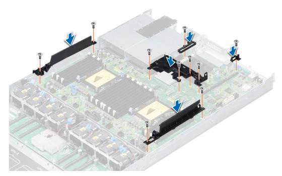
Figure 103. Installing the cable guides, NDC guide, PCIe guide, and PCH shroud base
