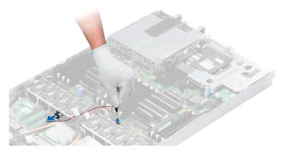
Figure 39. Removing the intrusion switch
