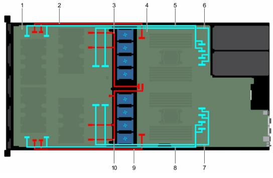
Figure 83. Configuration M: Cabling dual processor systems with SXM2 GPUs- direct connect
