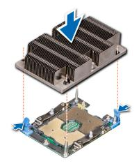
Figure 60. Installing a processor and heat sink module (1U)
