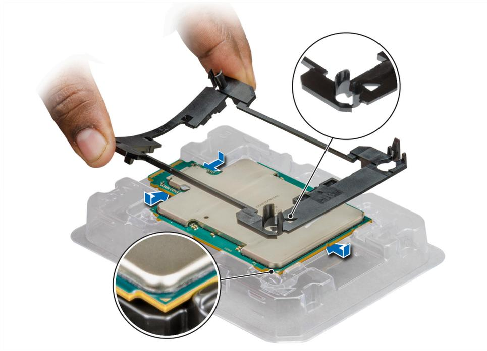
**Figure 33. Installing the processor bracket**
