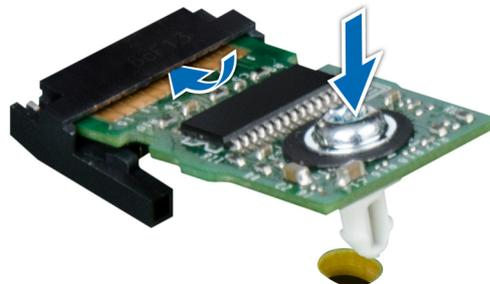
Figure 75. Installing the TPM
