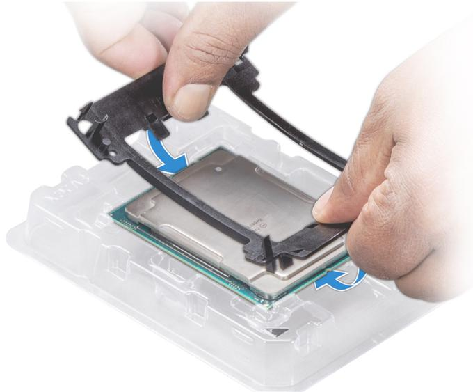
**Figure 40. Installing the processor bracket**
