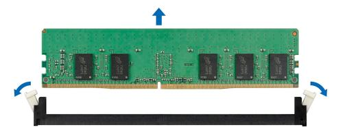
Figure 23. Removing a memory module
