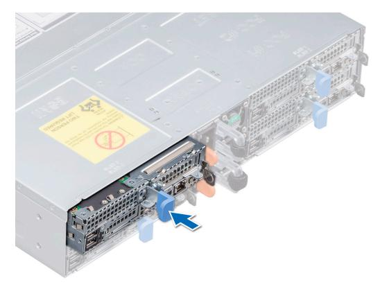
Figure 17. Stop the sled at a distance of 20-30 mm before complete insertion
