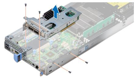
Figure 45. Removing the expansion card riser assembly
