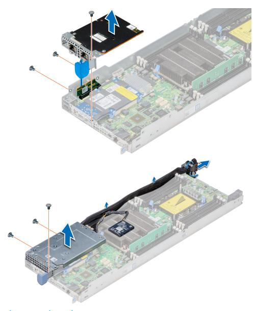
Figure 65. Removing a mezzanine card
