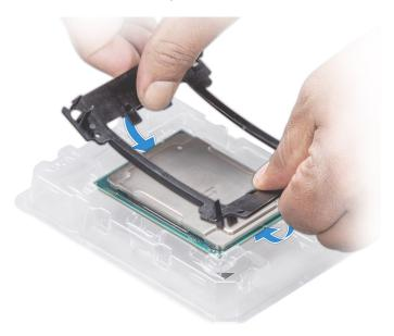
Figure 40. Installing the processor bracket
