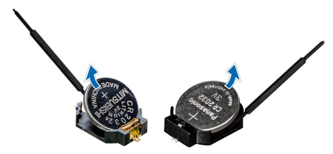
Figure 71. Removing system battery
