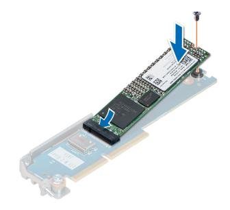
Figure 57. Installing the M.2 SATA card on the SATA x16 riser
