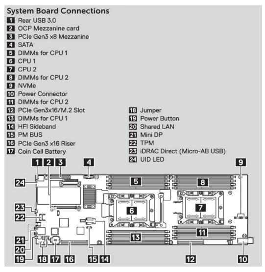
Figure 8. System board connections
