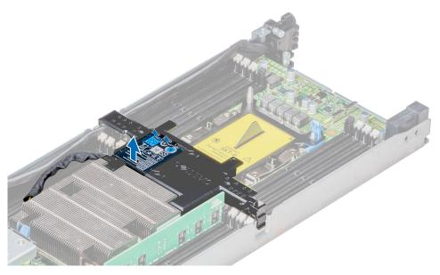
Figure 18. Removing the PERC battery
