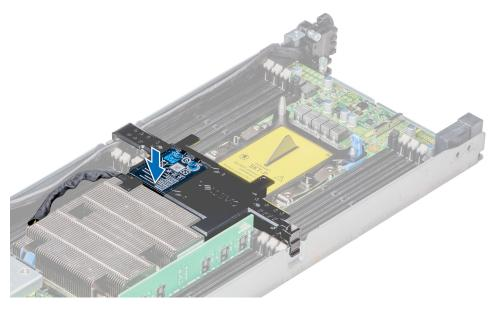
Figure 19. Installing the PERC battery
