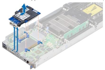
Figure 69. Removing the OCP card
