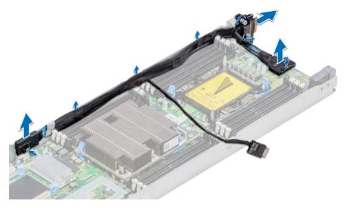
Figure 27. Removing the linking board and SATA cable
