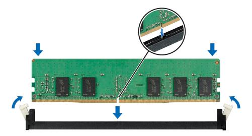
Figure 24. Installing a memory module
