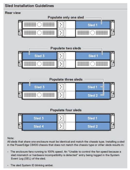
Figure 12. Sled Installation Guidelines
