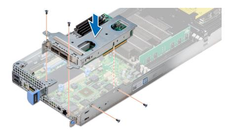
Figure 46. Installing the expansion card riser assembly
