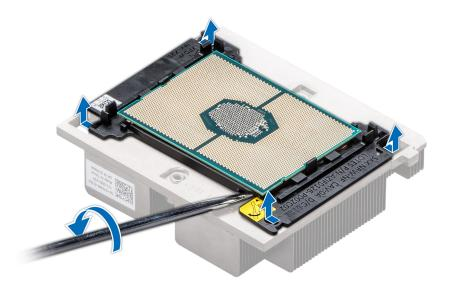
Figure 37. Loosening the processor bracket
