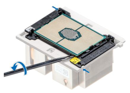
Figure 38. Loosening the processor bracket
