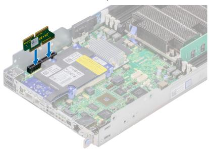
Figure 68. Installing the mezzanine card bridge board
