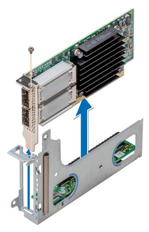
Figure 47. Removing an expansion card
