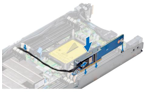
Figure 60. Installing the M.2 SATA x16 riser
