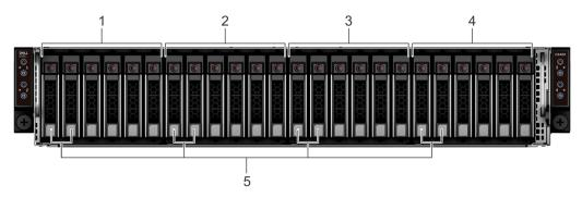
Figure 5. Sled to drive mapping for 24 x 2.5-inch drive configuration
