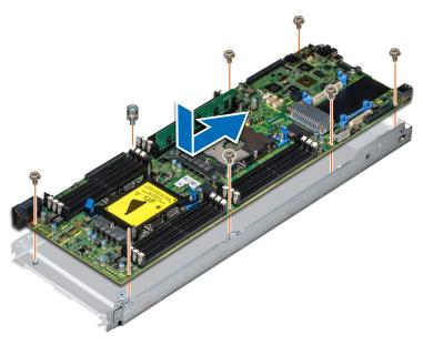
Figure 74. Installing system board
