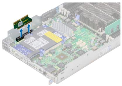
Figure 67. Removing the mezzanine card bridge board
