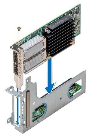
Figure 50. Installing an expansion card
