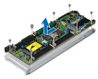
Figure 73. Removing the system board
