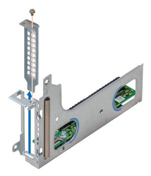
Figure 49. Removing the expansion card filler bracket
