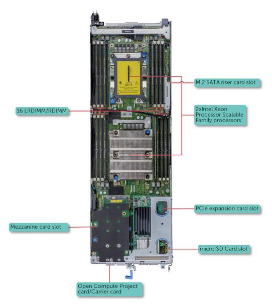
Figure 1. Supported configurations for PowerEdge C6420
