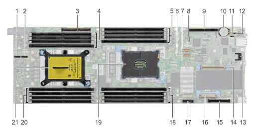
Figure 76. PowerEdge C6420 system board connectors
