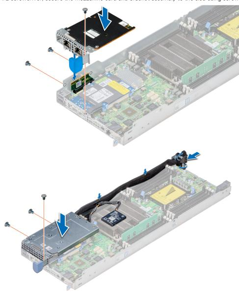
Figure 66. Installing a mezzanine card
