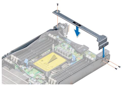
Figure 26. Installing the support bracket
