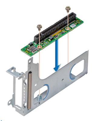
Figure 52. Installing the riser card
