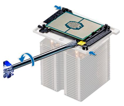
Figure 36. Loosening the processor bracket
