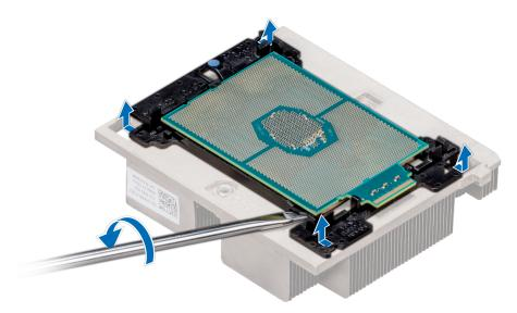
Figure 31. Loosening the processor bracket
