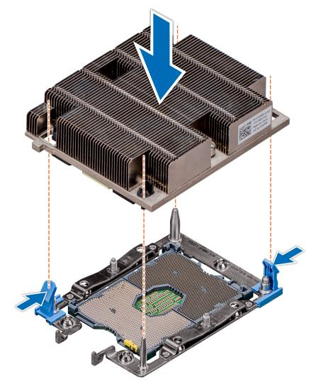
Figure 30. Installing a processor and heat sink module
