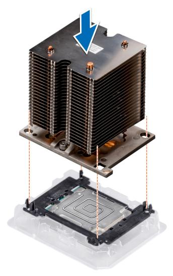
Figure 42. Installing the heat sink onto the processor
