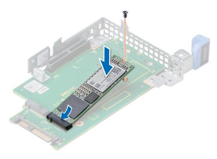
Figure 58. Installing the M.2 SATA card on the SATA x8 mezzanine card
