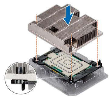
Figure 35. Installing the heat sink onto the processor
