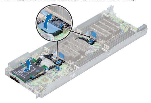
Figure 43. Removing the fabric and sideband cables
