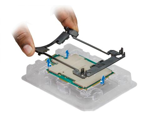
Figure 32. Removing the processor bracket
