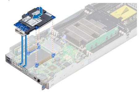
Figure 70. Installing the OCP card
