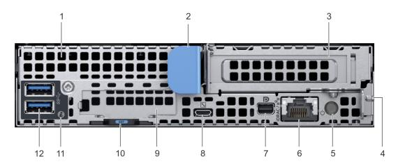
Figure 2. Back view of the PowerEdge C6420 sled
