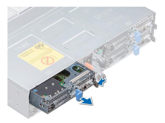
Figure 13. Removing a sled
