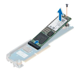
Figure 55. Removing the M.2 SATA card from the M.2 SATA x16 riser
