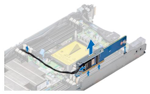
Figure 59. Removing the M.2 SATA x16 riser
