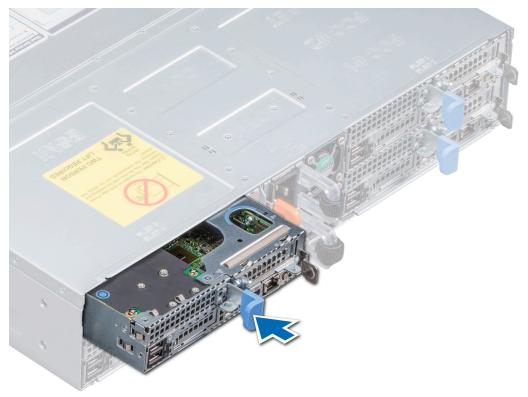
Figure 15. Installing a sled
