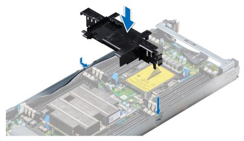
Figure 21. Installing the air shroud
