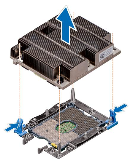
Figure 29. Removing the processor and heat sink module
