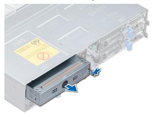
Figure 14. Removing a sled blank
