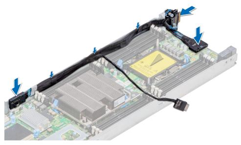
Figure 28. Installing the linking board and SATA cable
