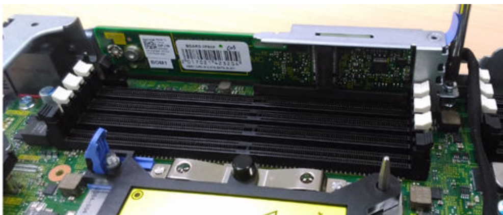
Figure 6. M.2 Boot Device installed in buried x16 PCIe slot
