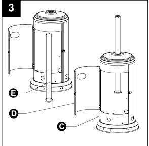
4. Secure post (E) to cylinder housing (C) using the reinforced ring (MM), M6 x 10 mm bolts (FF) and  $\Phi$ 6 small flat washers (GG). Fasten and cover with the deco ring (NN).
