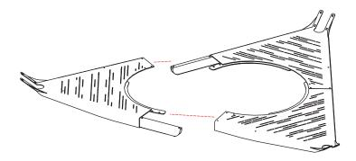
4 Tie the table pieces and the center hole support wings with six more 18mm M8 screws.
