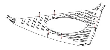
2 Carefully slide all 3 parts together, ensuring that the support tube and tabs nest properly.
