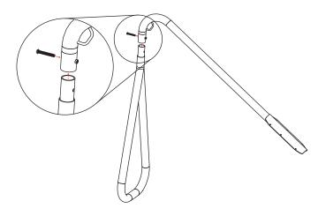
3 Slide the female end of the Lower arm tube onto the leg assembly. Insert and tighten 2 bolts into the lower set of holes on the reinforcement bracket. Repeat 3 times.
