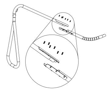
4 Insert the male end of all three leg assemblies into the 3 way center joint. Secure in place with the 60mm M8 Bolts.
