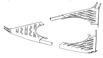
3 Secure the table to the welded support tubes with six 18mm M8 screws.
