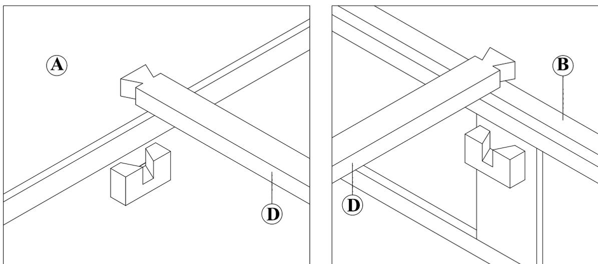
10. Attach Slats (I) to the whole body. Use the wood stopper to guide.
