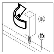
9. Attach Center Rail (D) with Extra Leg (E) to bed. Please DO NOT attach Center Rail (D) without first securing Extra Leg (E) to the whole body otherwise Center Rail (D) can break.
