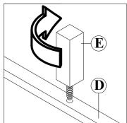
6. Attach Center Rail (D) with Extra Leg (E) to bed. Please DO NOT attach Center Rail (D) without first securing Extra Leg (E) to the whole body otherwise Center Rail (D) can break.
