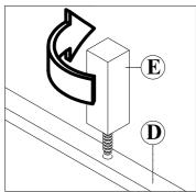
5. Attach Center Rail (D) with Extra Leg (E) to bed. Please DO NOT attach Center Rail (D) without first securing Extra Leg (E) to the whole body otherwise Center Rail (D) might break. ASSEMBLY IS COMPLETED
