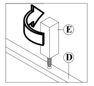
6. Attach Center Rail (D) with Extra Leg (E) to bed. Please DO NOT attach Center Rail (D) without first securing Extra Leg (E) to the whole body otherwise Center Rail (D) can break.
