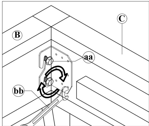
4. Make sure to tighten all bolts by using Wrench (bb).
