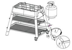
/ Position the stand with the castor wheels to the right. Two people should lift the barbeque and hood assembly (01A) by the serveries, and place it within the stand (facing forwards, castors to the right). Fix the barbeque to the stand top with the four M6x0.8in (20mm) screws and 0.2in (6mm) flat washers removed at step 2 – two to the front and two to the rear. Tighten fully.
