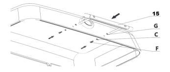
Angle the assembly slightly to the back and remove both M6x0.8in (20mm) screws, then do the same at the front, supporting the parts so they don't drop. Keep all of the fasteners for later use. Removable stickers at the front and rear will mark the positions of these screws. Remove the hood and barbeque chassis assembly from the stand top and place on the ground.
