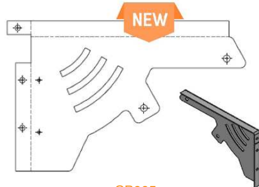
CR225 Combustible Wall Mounting Bracket Kit Surface area = 140.69 square inches
