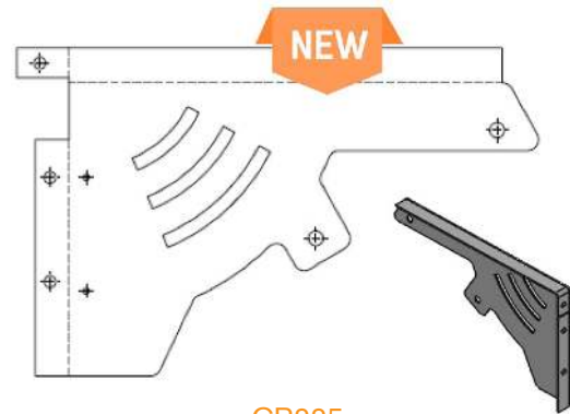
CR225 Combustible Wall Mounting Bracket Kit Surface area = 140.69 square inches
