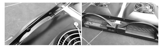
Position SS-UVB symetrically to mounted brackets and secure provided hanging clips with loop holes just inside brackets. Insert rivets through loop holes and then through holes at the ends of the brackets to complete mounting of UVB unit. The new bracket contains holes in the same position as the original bracket for inserting the original V hangers that came with the light fixture. This also applies to the SolarXtreme 1000.
