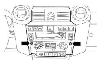
Step 5: Now with the centre dash removed, disconnect the connector from the back of the cigarette lighter. Connect the harness from your one touch indicator module in line with your cigarette lighter socket.
