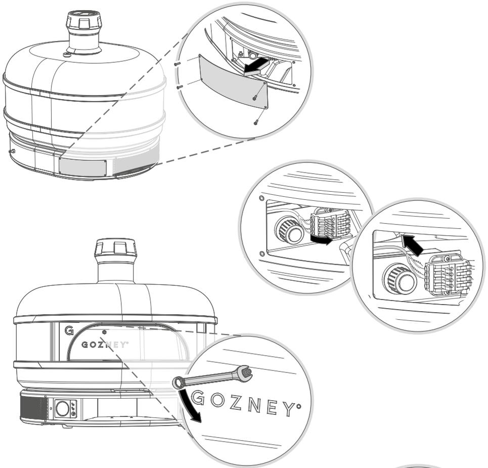
Only when the oven is cold, remove the rear panel to access the probe terminal. The terminal is held with a magnet so can be removed from the dock easily to gain better access. Lift all the levers on the left hand side of the terminal to release the probe wires. Unscrew the probe from inside the oven and pull the old probe out the mouth of the oven.
