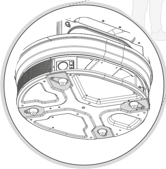
Never attempt to move the oven on your own. Two people should pick up the oven lifting from under the rounded ends of the oven, do not use the mouth of the oven as a lifting point.
