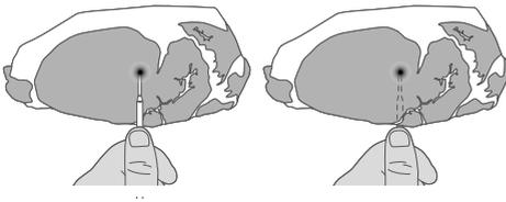
The coldest section of the meat will be in the centre of the thickest part. Placing the probe on top of the meat and using your thumb as a depth guide is the best way to ensure the probe is positioned correctly.
