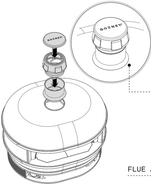
The flue is designed to have a rain guard which has a 5mm gap from the Dome.
