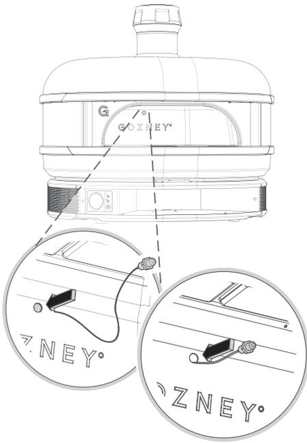
Push the new probe's wires into the hole and feed them through until they are visible from inside the rear panel. Hand tighten the probe in place, avoid using a spanner as you may damage the probe.
