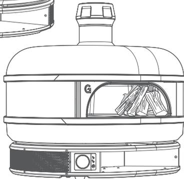
The flame from the wood fire should role across the length of the oven's roof. Avoid overfeeding the fire, there should never be flames coming out the mouth of the oven. If you are struggling to get a good flame ensure the wood you are using follows our guidelines at the beginning of this chapter.
