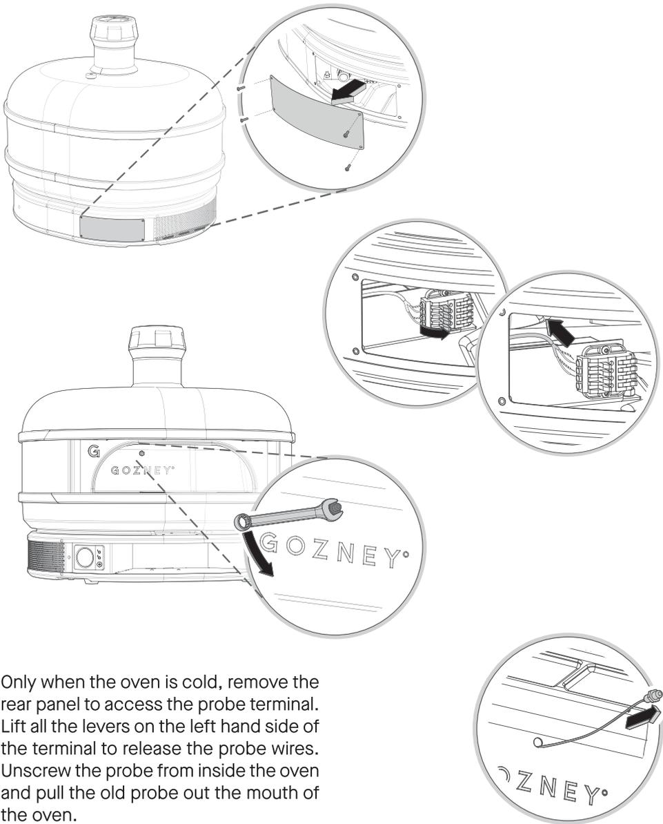
Only when the oven is cold, remove the rear panel to access the probe terminal. Lift all the levers on the left hand side of the terminal to release the probe wires. Unscrew the probe from inside the oven and pull the old probe out the mouth of the oven.
