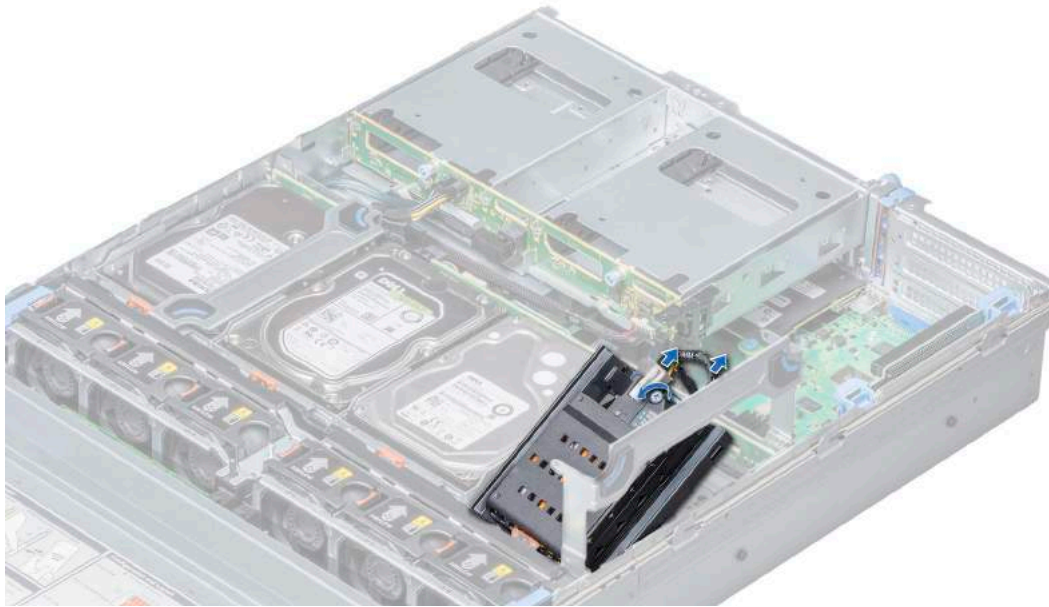
Figure 35. Removing NVDIMM-N battery from mid drive tray
