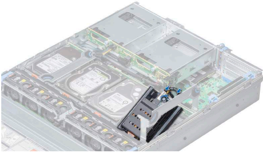
Figure 36. Installing NVDIMM-N battery into mid drive tray
