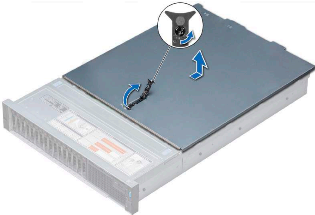
Figure 19. Removing the system cover
