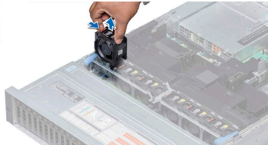
Figure 29. Removing cooling fan
