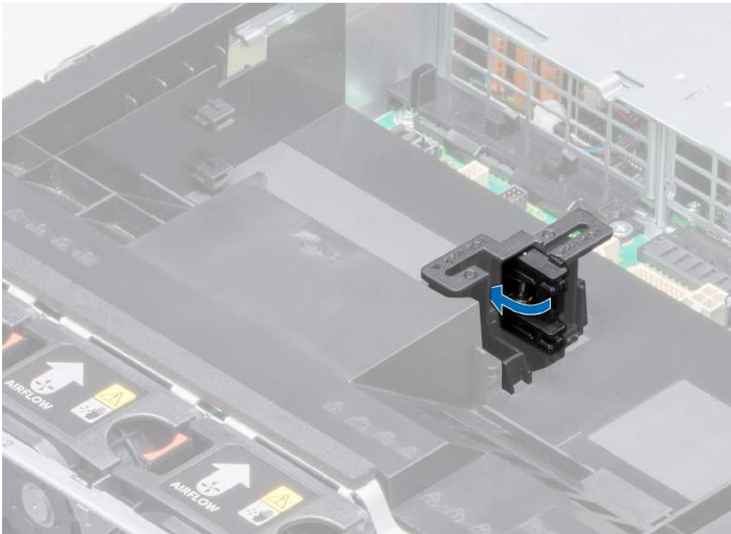
Figure 72. Closing the PCIe card holder latch
