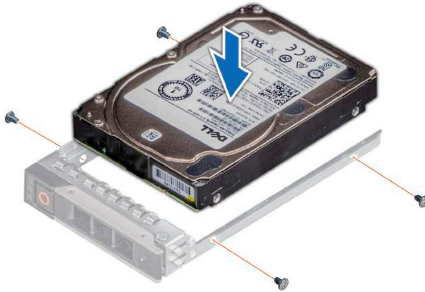
Figure 54. Installing a drive into the drive carrier
