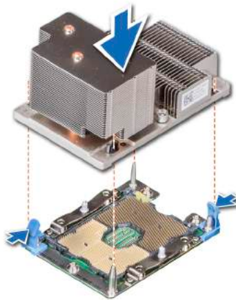
Figure 69. Installing the processor and heat sink module (2U)
