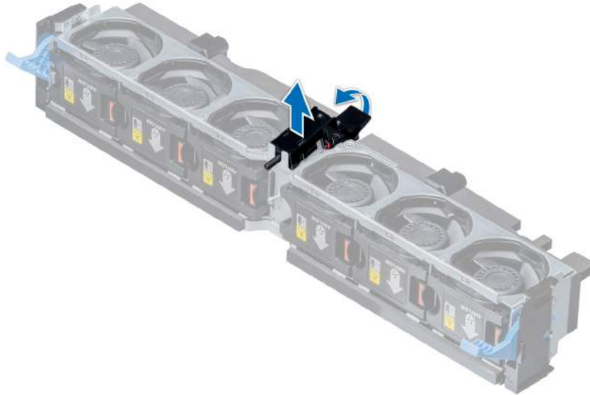
Figure 31. Removing an intrusion switch
