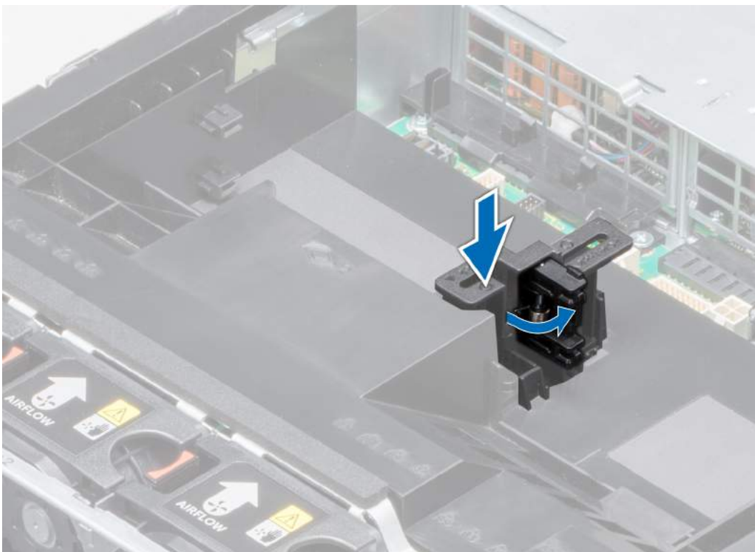
Figure 71. Opening the PCIe card holder latch
