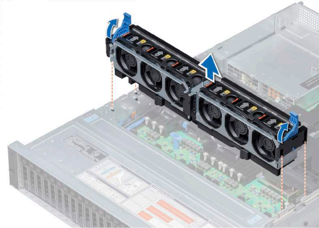
Figure 27. Removing the cooling fan assembly
