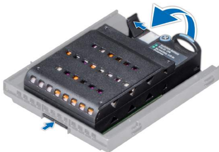
Figure 37. Removing NVDIMM-N battery from the bracket
