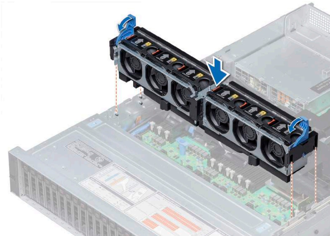
Figure 28. Installing the cooling fan assembly
