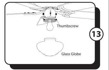
13. Loosen the three thumbscrews near the bottom of the light kit. Lift the glass globe into the light kit and retighten the previously loosened thumbscrews to secure.
