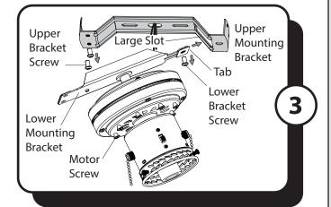
3. Remove the preassembled lower bracket screw from the lower mounting bracket and the upper bracket screws from the upper mounting bracket. Remove the motor screws and set aside for later. Place one tab of the lower bracket into a large slot in the upper mounting bracket.
