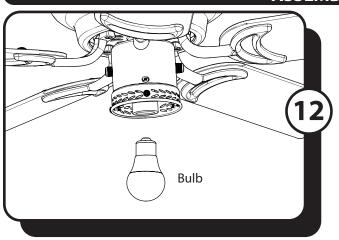
12. Install the E26-base LED bulb in the socket. **Important:** Make sure you allow the bulbs and light kit to cool before you replace the bulbs.
