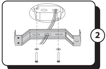
2. Secure the upper mounting bracket to the outlet box using screws, spring washers, provided with the outlet box (not included).
