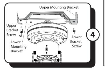
4. Reinstall the previously removed lower bracket screw and upper mounting screws to secure the lower mounting bracket to the upper mounting bracket.
