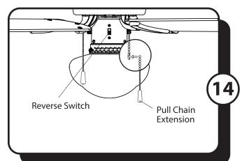
14. Attach the pull chain extensions to the fan and light pull chains.
