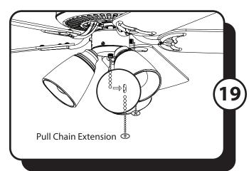
19. Attach pull chain extensions to the pull chains. **Note:** The pull chain in the center of the light kit controls the light.
