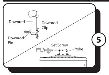
5. **DOWNROD MOUNT** - Remove the downrod clip and downrod pin from the downrod. Then, loosen but don't remove the two set screws at the top of the yoke.
