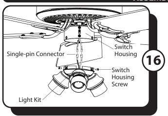
16. Remove the three switch housing screws from the top edge of the light kit. Then, connect the single-pin connectors from the switch housing to the single-pin connectors from the light kit -- blue to blue and white to white.
