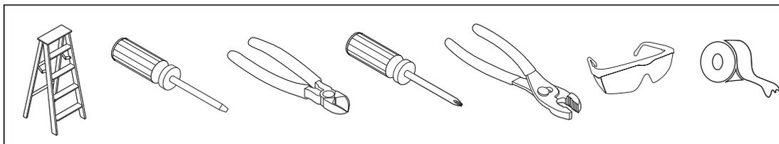
**Tools required for assembly:** Electrical tape, Phillips Screwdriver, Pliers, Safety Glasses, Step Ladder, Wire Cutters and Wire Strippers
