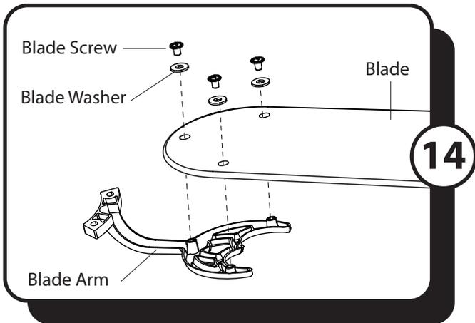
14. Partially insert three blade screws along with three blade washers through one blade and into one blade arm. Tighten each blade screw with a Phillips screwdriver (not included), starting with the one in the middle. Repeat this step for the remaining blades and blade arms.
