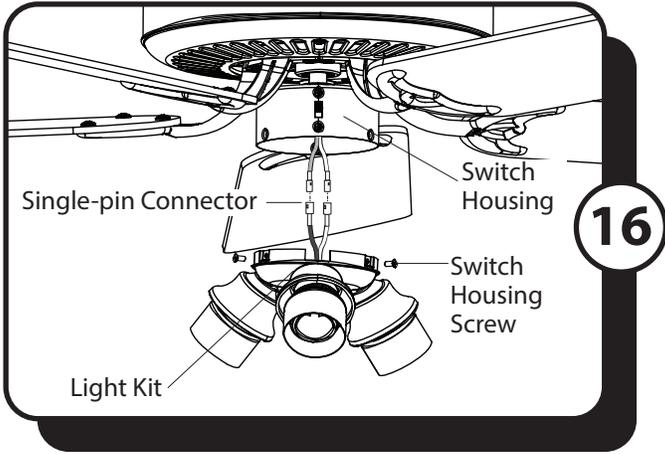
16. Remove the three switch housing screws from the top edge of the light kit. Then, connect the single-pin connectors from the switch housing to the single-pin connectors from the light kit -- blue to blue and white to white.
