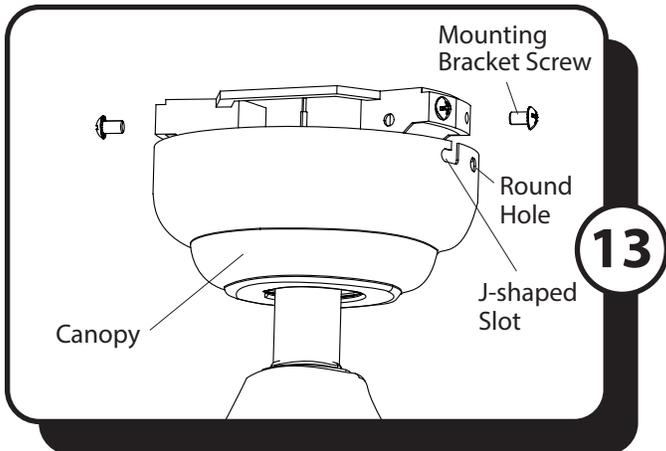
13. Align the canopy over the loosened mounting bracket screws. Place the J-slot of the canopy onto the mounting bracket screws and rotate clockwise. Secure the canopy with the two previously removed mounting bracket screws. Tighten all the mounting bracket screws securely.
