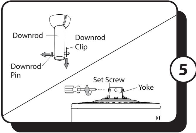
5. **DOWNROD MOUNT** - Remove the downrod clip and downrod pin from the downrod. Then, loosen but don't remove the two set screws at the top of the yoke.
