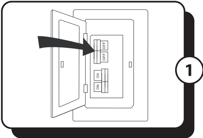
1. Turn **OFF** the electrical power at the main fuse or circuit breaker.
