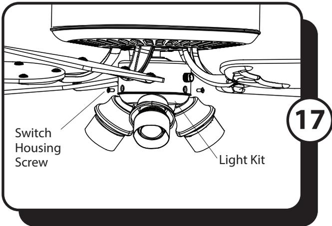
17. Use the three previously removed switch housing screws to secure the light kit to the switch housing.
