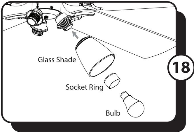
18. Remove the socket ring from each socket. Raise the glass shade over the socket of the light kit. Secure the glass shade by twisting the socket ring clockwise onto the socket. Repeat for each socket. Install the E26-base LED bulbs into the sockets in the light kit.
