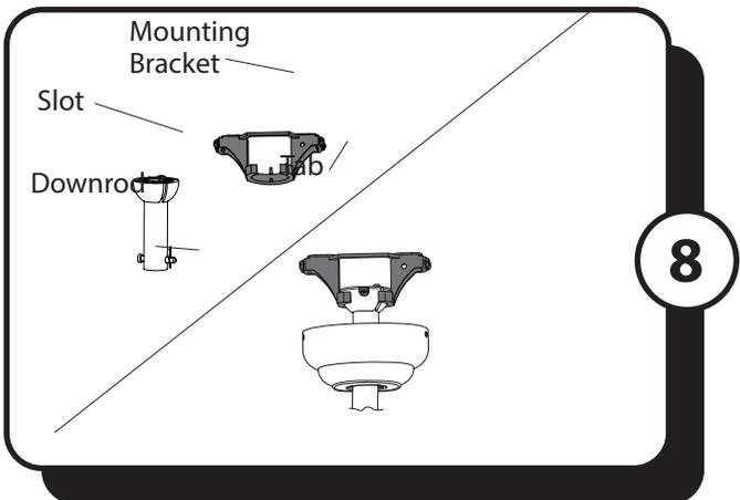
8. Lift the downrod into the mounting bracket. Rotate the downrod until the tab in the mounting bracket is seated in the slot in the downrod ball.
