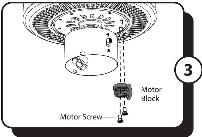
3. Remove the ten motor screws and five motor blocks from the underside of the motor assembly. Discard the motor blocks, but keep the motor screws for later.
