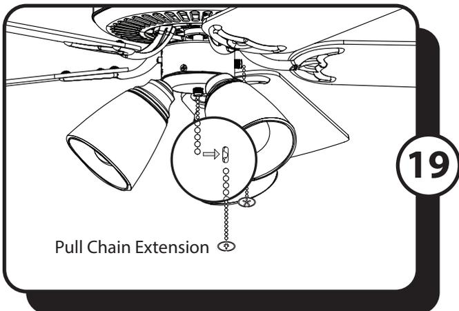
19. Attach pull chain extensions to the pull chains.
