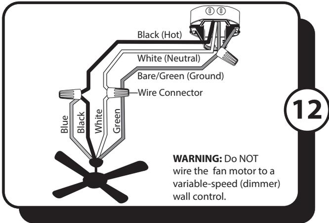
12. Use wire connectors to connect the fan wires to the power supply wires according to the wiring diagram and the following instructions:
