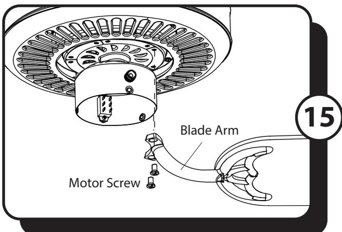
15. Install the blade arm to the underside of the motor assembly with previously removed motor screws. Tighten each blade arm completely before moving to the next.
