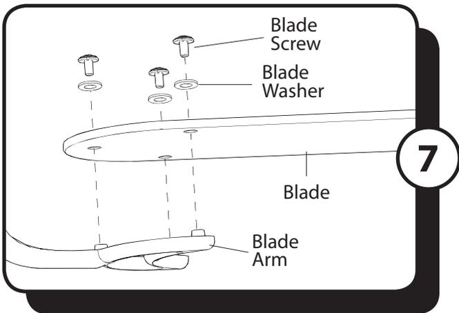
7. Partially insert the blade screws along with the blade washers through the blade and into the blade arm. Tighten each blade screw with a Phillips screwdriver starting with the one in the middle. Repeat this step for the remaining blades and blade arms.
