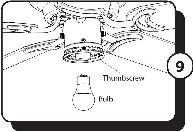
9. Install the E26-base LED bulb. Then, loosen the three thumbscrews on the lower edge of the light kit.
