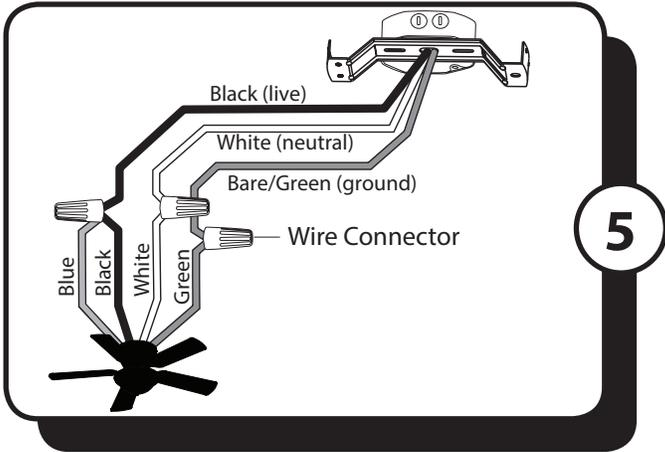
5. Use wire connectors to connect the fan wires to the power supply wires according to the wiring diagram and the following instructions:
