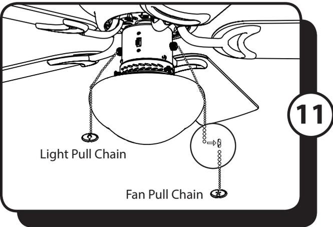
11. Attach the pull chain extensions to the fan and light pull chains. When facing the reverse switch, the light pull chain is on the left and the fan pull chain is on the right.
