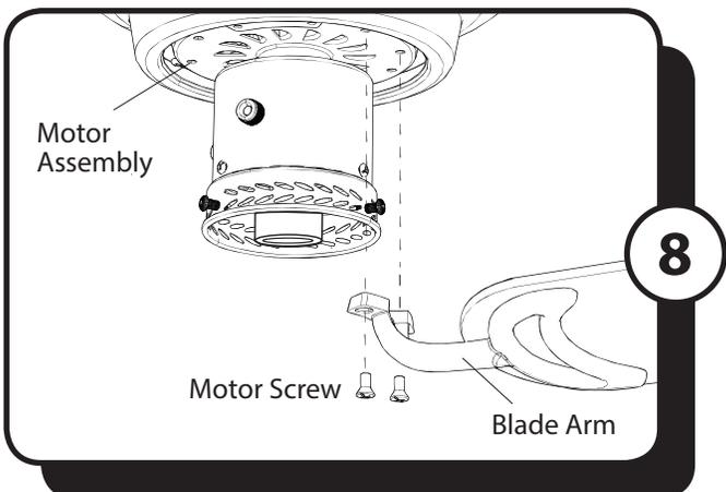
8. Remove the ten motor screws from the underside of the motor assembly. Secure each blade arm to the underside of the motor assembly using two previously removed motor screws. Completely secure each blade arm before moving to the next.
