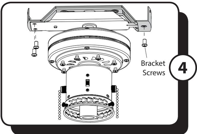
4. Secure the lower bracket to the mounting bracket with the three previously removed bracket screws.
