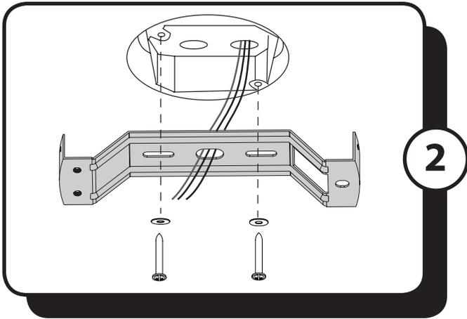
2. Secure the mounting bracket to the outlet box (not included) using the two mounting screws supplied with outlet box.
