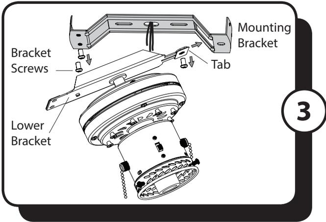
**Note:** Remove the wire restraint from the wires on top of the lower bracket.
