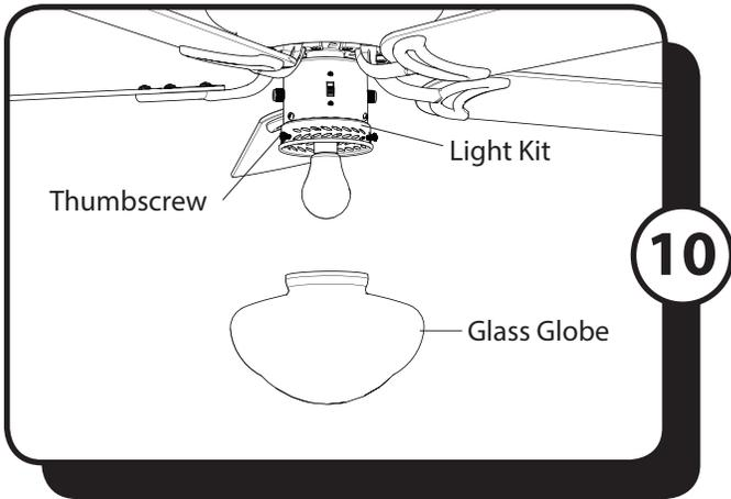
10. Lift the glass globe to light kit, secure by tightening the loosened thumbscrews.
