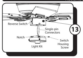
13. Remove the three switch housing screws from the light kit. Then, connect the single-pin connectors from the switch housing to the light kit -- white to white and blue to black.
