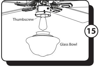
15. Loosen the three thumbscrews at the bottom edge of the light kit. Lift the glass bowl into the light kit and hand tighten the thumbscrews to secure the glass bowl.
