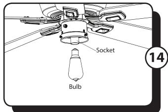
14. Install the E26-base LED bulb into the socket of the light kit.
