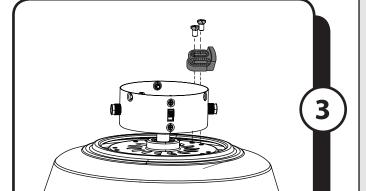
3. Remove the 10 motor screws and five motor blocks from the underside of the motor assembly. Discard the motor blocks, but keep the motor screws for later.
