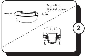
2. Remove the canopy from the mounting bracket by removing the two mounting bracket screws from the round holes in the canopy. Then loosen the other two mounting bracket screws from the J-shaped slots. Retain the mounting bracket screws for later. Install the mounting bracket to the outlet box (not included) using the screws and washers provided with the outlet box.
