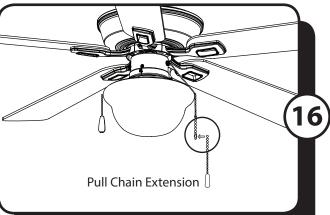
16. Attach the pull chain extension(s) to the pull chain(s).
