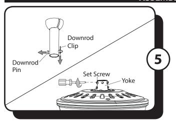
5. **DOWNROD MOUNT** - Remove the downrod pin and downrod clip from the downrod. Then, loosen but do not remove the two set screws in the yoke.
