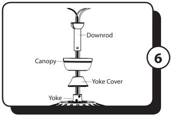
6. Feed the wires coming from the yoke through the yoke cover, canopy and downrod.
