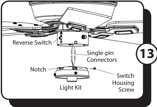
13. Remove the three switch housing screws from the light kit. Then, connect the single-pin connectors from the switch housing to the light kit -- white to white and blue to black.
