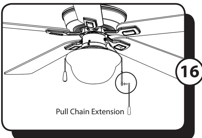
16. Attach the pull chain extension(s) to the pull chain(s).
