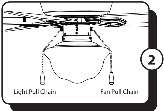
2. The fan pull chain has four positions to control fan speed. One pull is HIGH, two is MEDIUM, three is LOW and four turns the fan OFF.
