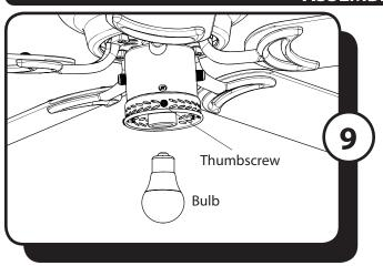
9. Install the E26-base LED bulb. Then, loosen the three thumbscrews on the lower edge of the light kit.
