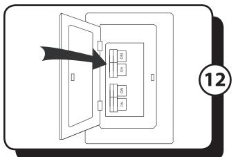
12. Restore the power at the main fuse or circuit breaker.
