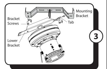
**Note:** Remove the wire restraint from the wires on top of the lower bracket.
