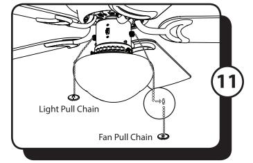
11. Attach the pull chain extensions to the fan and light pull chains. When facing the reverse switch, the light pull chain is on the left and the fan pull chain is on the right.
