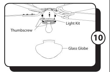
10. Lift the glass globe to light kit, secure by tightening the loosened thumbscrews.
