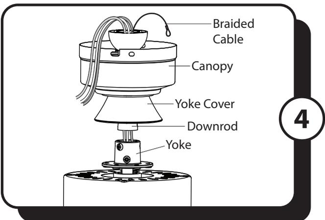
4. Feed the wires and braided cable coming from the yoke through the yoke cover, canopy and downrod.
