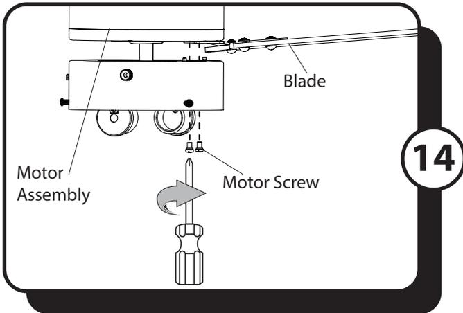
14. Attach a blade assembly to the underside of motor assembly using previously removed motor screws. Completely secure each blade assembly before moving to the next.
