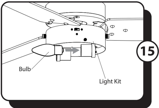
15. Install the bulbs into the sockets of the light kit. **Important:** Make sure to allow the bulbs to cool before you replace them.
