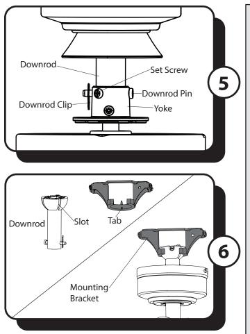
5. Insert the downrod into the yoke and reinstall the downrod pin and downrod clip. Then retighten the two set screws.
