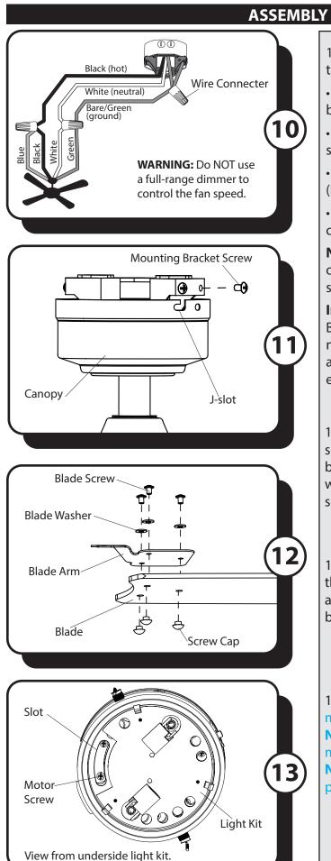
10. Connect household supply and fan wires according to the diagram and these steps:
