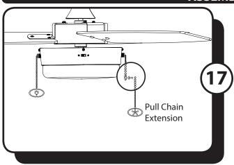
17. Attach the pull chain extensions to each of the pull chains.
