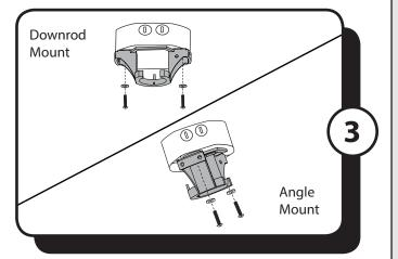
3. Attach mounting bracket to outlet box (not included) using screws and washers provided with the outlet box.
