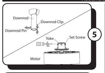
5. Remove the downrod clip and downrod pin from the downrod. Then partially loosen the two set screws in the yoke at the top of the motor.
