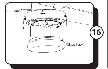
16.. Lift the glass bowl up to the light kit and turn in a clockwise direction until it is secure.
