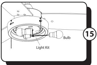
15. Install the E26-base, A15 LED bulbs into the sockets of the light kit.
