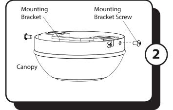
2. Loosen all mounting brackets screws. Remove the two mounting bracket screws from the round holes of canopy. Set aside for later use. Detach mounting bracket from canopy.
