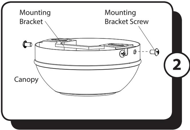
2. Loosen all mounting brackets screws. Remove the two mounting bracket screws from the round holes of canopy. Set aside for later use. Detach mounting bracket from canopy.
