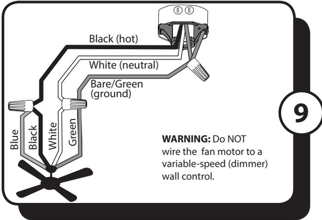
9. Use wire connectors to connect the fan wires to the power supply wires according to the wiring diagram and the following instructions:
