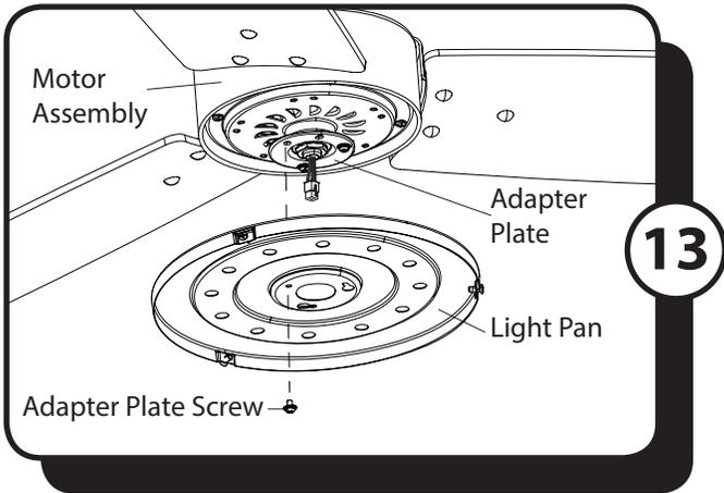
13. Remove one of the three adapter plate screws from the adapter plate and loosen the other two screws, but do not remove. Align the keyholes of the light pan with the loosened adapter plate screws, then turn the light pan in a clockwise direction. Replace previously removed adapter plate screw, then tighten all screws.
