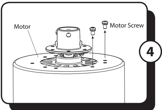
4. Remove the six Phillips-head motor screws from the top of the motor. Save screws for blade arm attachment.
