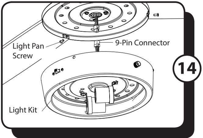
14. Remove the three light pan screws from the light pan. Then, connect the 9-pin connector from the adapter plate to the 9-pin connector in light kit. Secure the light kit to the light pan using the three previously removed light pan screws.
