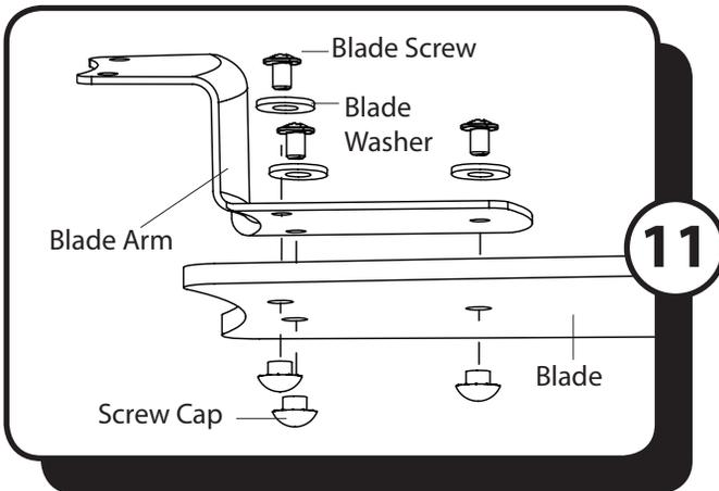
11. Insert the blade screws along with the blade washers through the blade arm and the blade and secure with a screw cap. Repeat this step for the remaining blades and blade arms.
