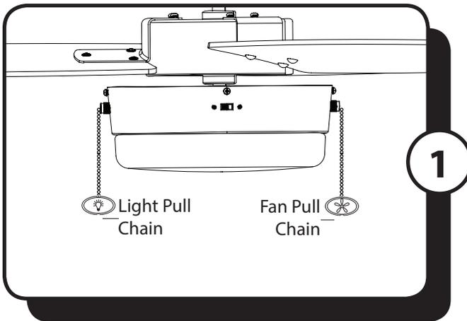
1. The fan pull chain is located to the right of the reverse switch. It has four positions to control fan speed. One pull is HIGH, two is MEDIUM, three is LOW and four turns the fan OFF. The light pull chain is located to the left of the reverse switch. It turns the light ON and OFF.
