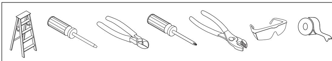
**Tool required for assembly:** Electrical tape, Phillips Screwdriver, Pliers, Safety Glasses, Step Ladder, Wire Cutters and Wire Strippers
