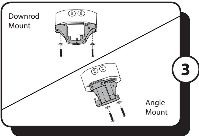
3. Attach mounting bracket to outlet box (not included) using screws and washers provided with the outlet box.
