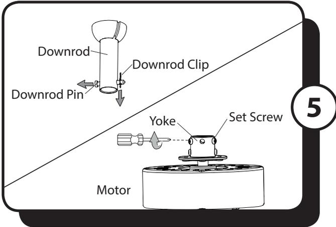
5. Remove the downrod clip and downrod pin from the downrod. Then partially loosen the two set screws in the yoke at the top of the motor.
