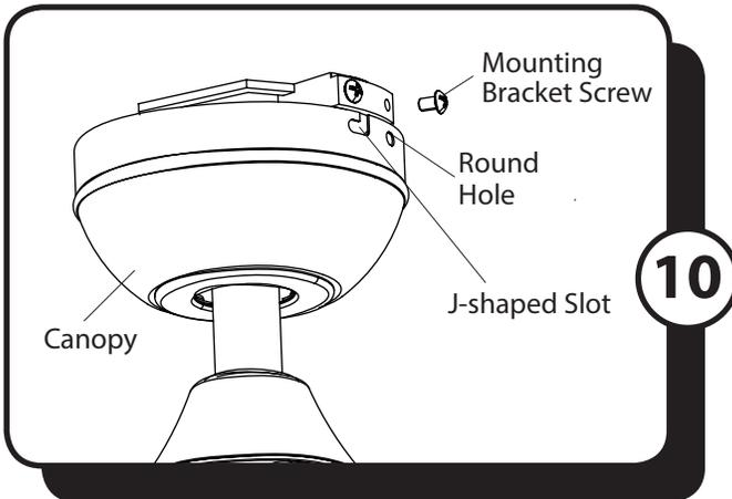
10. Raise the canopy, ensure the two mounting bracket screws are aligned with the J-shaped slots in the canopy. Then turn the canopy in a clockwise direction until the mounting bracket screws are completely engaged in the J-shaped slots. Install the two previously removed mounting bracket screws in the round holes. Securely tighten all four mounting bracket screws.
