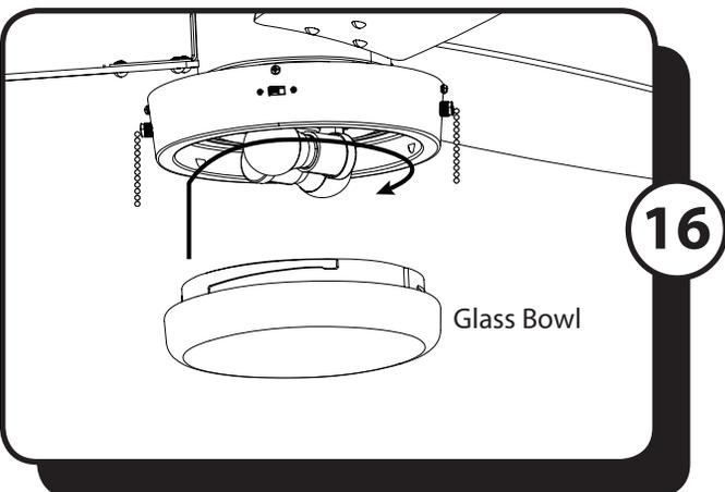
16. Lift the glass bowl up to the light kit and turn in a clockwise direction until it is secure.
