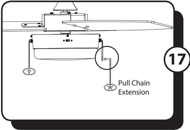
17. Attach the pull chain extensions to each of the pull chains.
