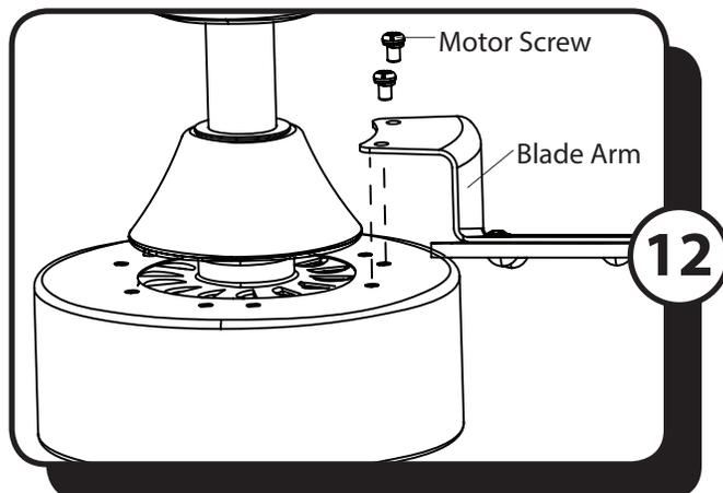
12. Secure the blade arm to the top side of the motor using the previously removed motor screws. Completely secure each blade arm to motor before moving to the next.
