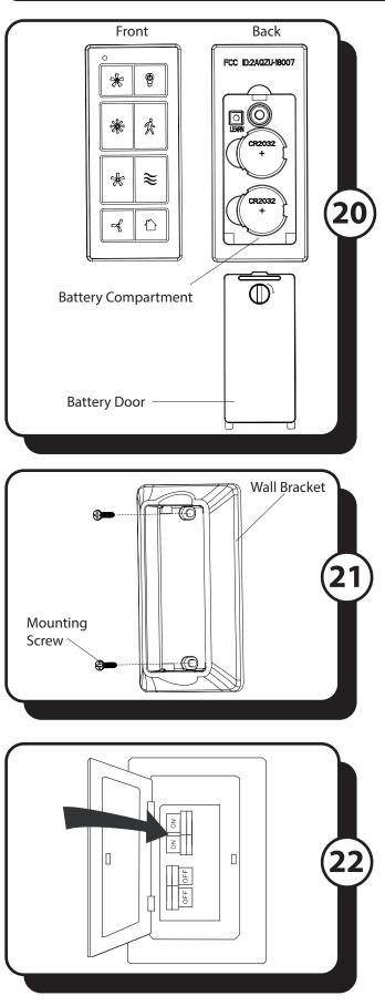
20. Remove the battery door from the back of the remote using a flat-head screwdriver (not included). Insert the two CR2032 batteries into the remote; ensure the positive pole of the batteries face up (as pictured) and then replace the battery door.
