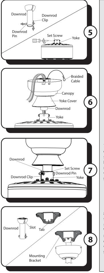
5. **DOWNROD MOUNT** - Remove the downrod clip and downrod pin from the downrod. Then, loosen but do not remove the two set screws at the top of the yoke.
