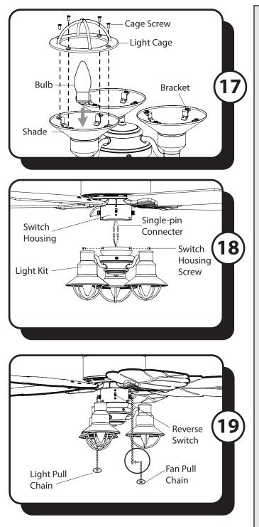
17. Remove the four cage screws from the brackets inside the shade. Install the E26-base LED bulb in the socket. Then attach the light cage to the shade using the four cage screws. Repeat for each shade.
