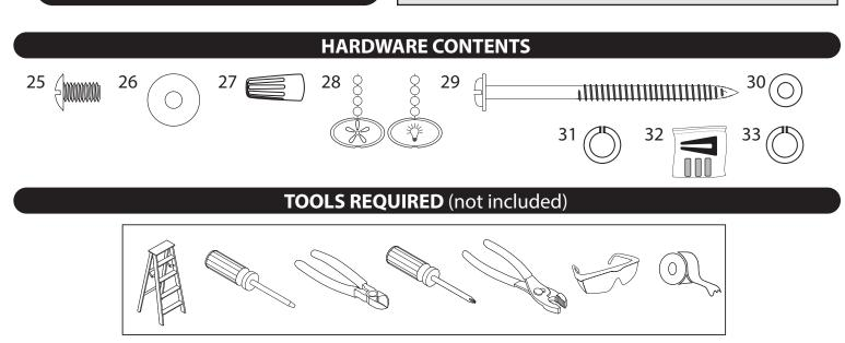
**Tools required for assembly:** Electrical tape, Phillips Screwdriver, Pliers, Safety Glasses, Step Ladder, Wire Cutters and Wire Strippers
