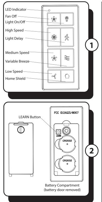
1. To operate the fan using the remote, make sure fan pull chain is on high and light is turned on. Then press and release the following buttons:
