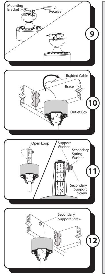
9. Place the receiver in the mounting bracket with flat side up to prepare for the wiring process.
