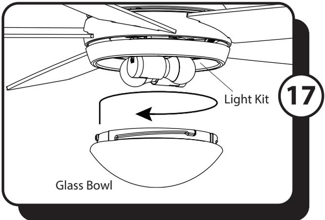
17. Attach the glass bowl to the light kit by twisting the glass bowl tightly in a clockwise direction until it is secure.
