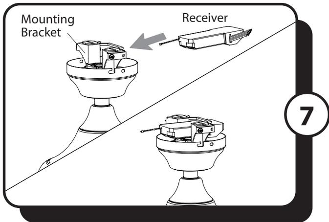
7. Insert the receiver from remote pack into the mounting bracket with antenna end first and the flat side facing the ceiling.
