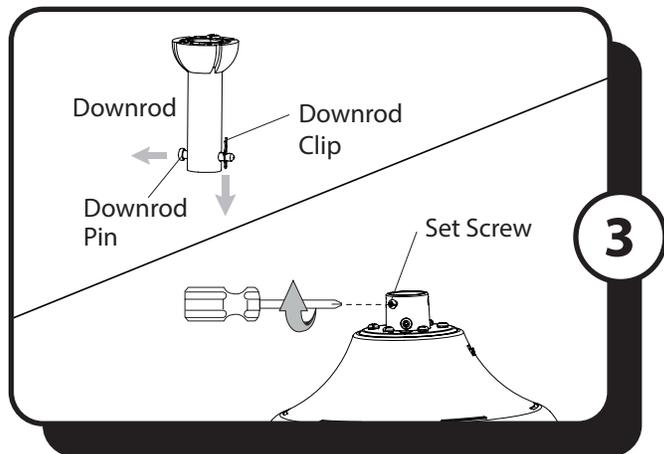
3. **Downrod Installation** - Remove the downrod clip and downrod pin from the downrod. Then, loosen but do not remove the two set screws at the top of the motor assembly.
