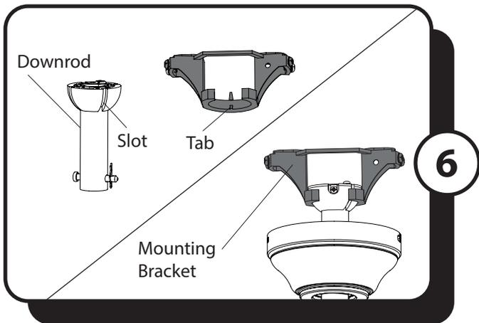
6. Install the ball end of the downrod into the opening of the mounting bracket. Rotate the downrod until the tab in the mounting bracket is seated in the slot in the downrod ball.
