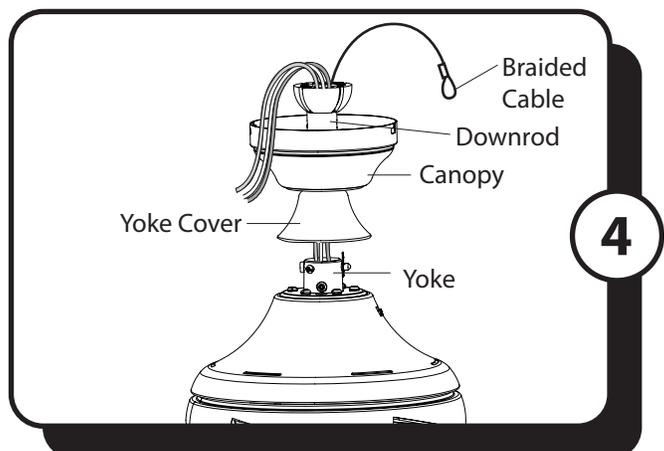
4. Insert the downrod through the canopy and yoke cover. Feed the wires and braided cable from the fan through the downrod.
