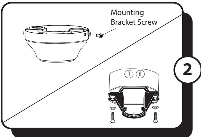
2. Loosen all four mounting bracket screws and completely remove the two screws from the round holes in the canopy. Then remove mounting bracket from the canopy and save them for later. Remove the canopy from the mounting bracket. Install the mounting bracket to the outlet box (sold separately) using the screws and washers provided with the outlet box.
