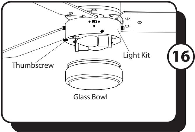
16. Loosen the three thumbscrews near the bottom of the light kit. Lift the glass bowl into the light kit and re-tighten the previously loosened thumbscrews to secure.
