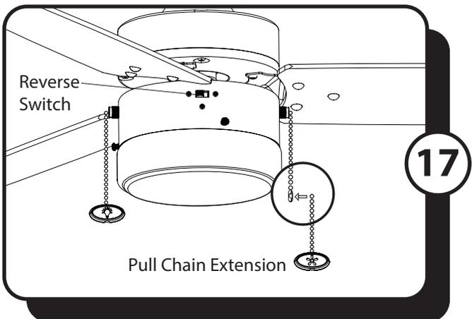
17. Attach pull chain extensions to the pull chains. **Note:** When facing the reverse switch, the fan pull chain is on the left and the light pull chain is on the right.
