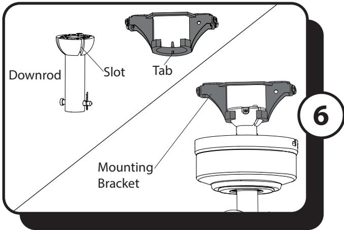
6. Lift the downrod into the mounting bracket. Rotate the downrod until the tab in the mounting bracket is seated in the slot in the downrod ball.
