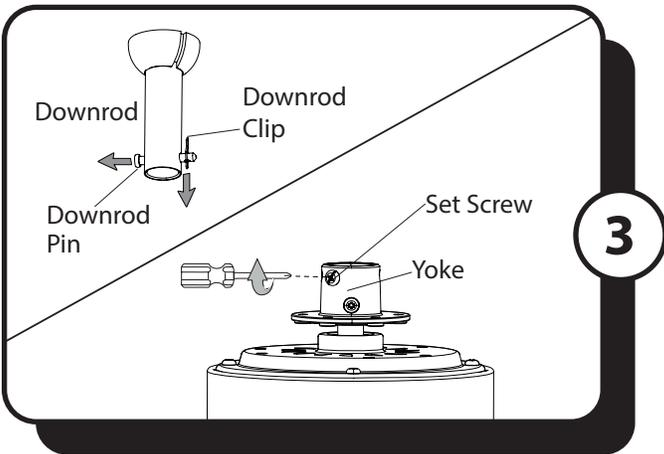
3. Remove the downrod clip and downrod pin from the downrod. Then, loosen but do not remove the two set screws at the top of the yoke.
