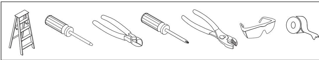
**Tools required for assembly:** Electrical tape, Phillips Screwdriver, Pliers, Safety Glasses, Step Ladder, Wire Cutters and Wire Strippers
