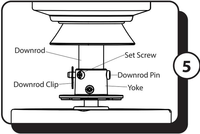
5. Insert the downrod into the yoke and reinstall the downrod pin and downrod clip. Then retighten the two set screws.
