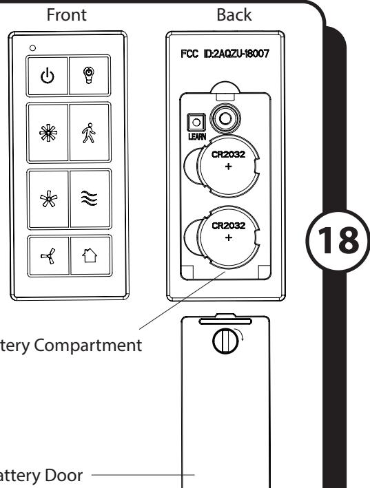
18. Remove the battery door from the back of the remote using a flat-head screwdriver (not included). Insert the two CR2032 batteries into the remote; ensure the positive pole of the batteries face up (as pictured) and then replace the battery door.
