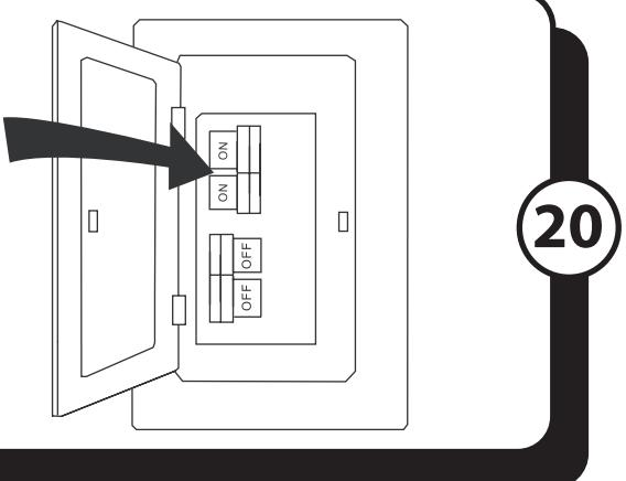
20. Turn ON the electrical power at the main fuse or circuit breaker and the wall switch.
