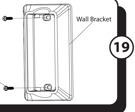
19. If desired, the wall bracket can be installed to the wall using the two mounting screws. Store the remote in the wall bracket when not in use.
