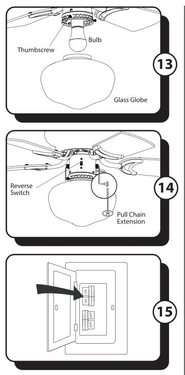
13. Install the E26-base LED bulb into the socket of the light kit. Then, loosen the three thumbscrews near the bottom of the light kit. Lift the glass bowl into the light kit and retighten the previously loosened thumbscrews to secure.
