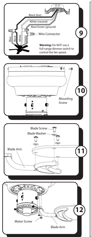
9. Use wire connectors to connect the fan wires to the power supply wires according to the wiring diagram and the following instructions:
