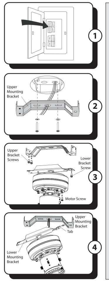
1. Turn **OFF** the electrical power at the main fuse or circuit breaker.
