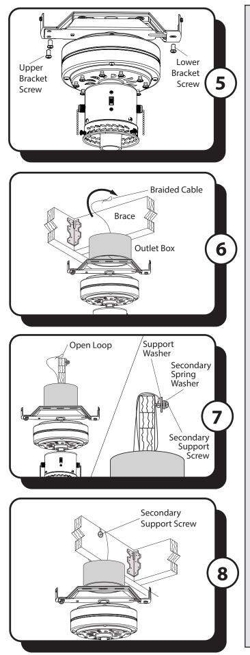
5. Reinstall the previously removed lower bracket screw and upper mounting screws to secure the lower mounting bracket to the upper mounting bracket.
