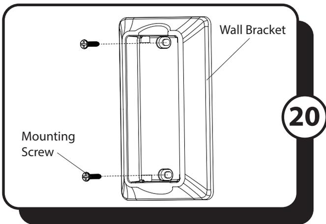
20. If desired, the wall bracket can be installed to the wall using the two mounting screws. Store the remote in the wall bracket when not in use.
