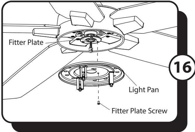
16. Remove one of the three fitter plate screws preassembled to the fitter plate and loosen the other two but do not remove. Feed the 9-pin connector through center hole in light pan. Align the slotted holes in the light pan with the loosened screws in the fitter plate. Turn light pan clockwise and replace the previously removed fitter plate screw. Tighten all screws.
