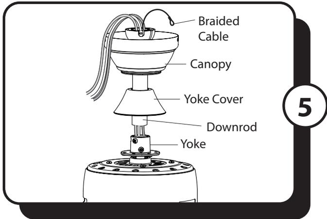
5. Insert the downrod through the canopy and yoke cover. Feed the wires and braided cable from the fan through the downrod.
