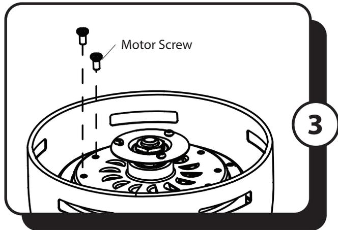
3. Remove the ten motor screws from the underside of the motor assembly. Save motor screws for later.
