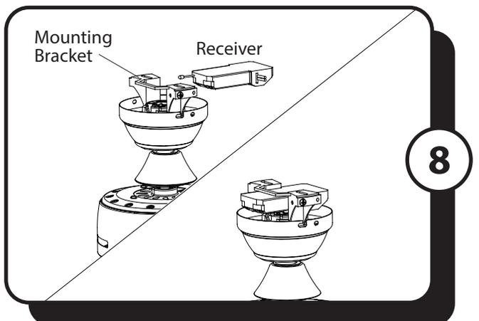
8. Insert the receiver, antenna first, into the mounting bracket with the flat side facing the ceiling.
