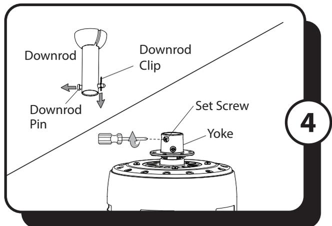
4. Remove the downrod clip and downrod pin from the downrod. Then loosen but do not remove the two set screws in the yoke at the top of the motor assembly.
