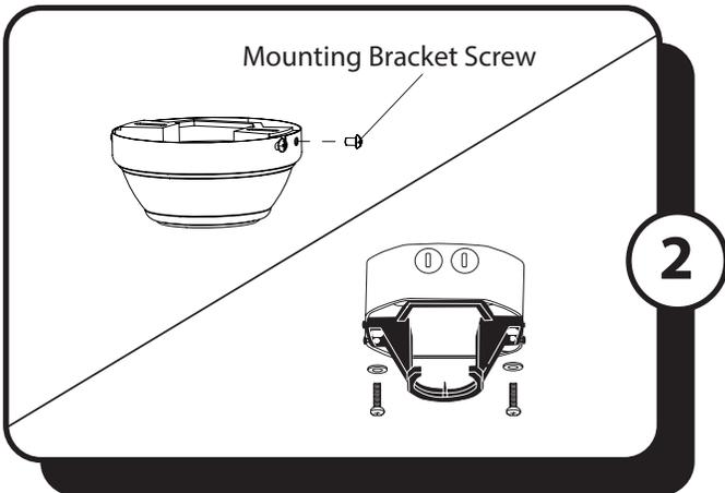
2. Remove the mounting bracket by removing the two mounting bracket screws from the round holes in the canopy. Then loosen the other two mounting bracket screws from the J-shaped slots. Retain the mounting bracket screws for later. Install the mounting bracket to the outlet box (not included) using the screws and washers provided with the outlet box.
