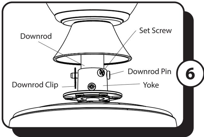
6. Slide the downrod into the yoke of the motor assembly, align the holes, then re-install the downrod pin and downrod clip. Secure with the two set screws and slide the yoke cover down until it rests on top of the motor assembly.
