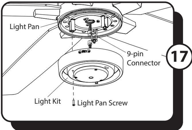
17. Remove one of the three light pan screws preassembled to the light pan and loosen the other two but do not remove. Connect the 9-pin connectors from the light pan to the 9-pin connectors from the light kit. Lift the two keyhole slots in the light kit over the two loosened light pan screws and turn in a clockwise direction. Then, use the previously removed light pan screw to secure the light kit to the light pan. Tighten all screws.
