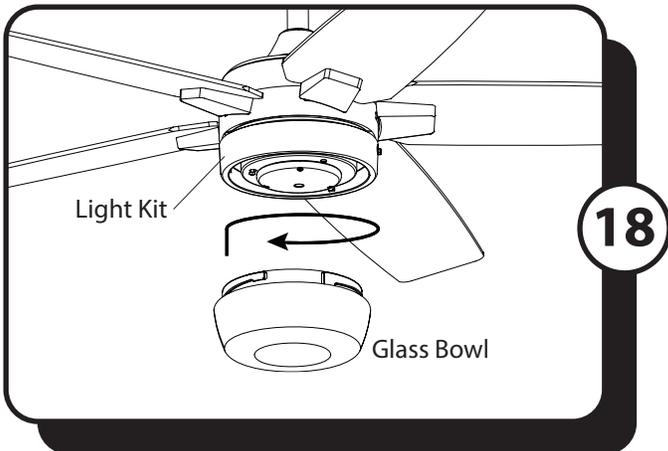
18. Attach the glass bowl to the light kit by twisting the glass bowl tightly in a clockwise direction until it is secure.
