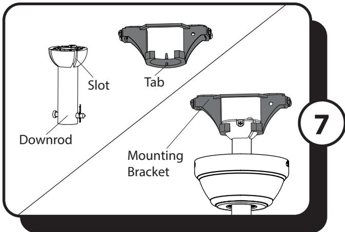
7. Install the ball end of the downrod into the opening of the mounting bracket. Rotate the downrod until the tab in the mounting bracket is seated in the slot in the downrod ball.
