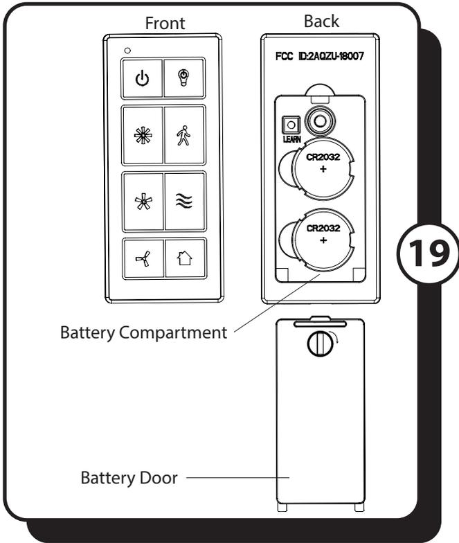
19. Remove the battery door from the back of the remote using a flat-head screwdriver (not included). Insert the two CR2032 batteries into the remote; ensure the positive pole of the batteries face up (as pictured) and then replace the battery door.
