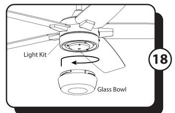
18. Attach the glass bowl to the light kit by twisting the glass bowl tightly in a clockwise direction until it is secure.
