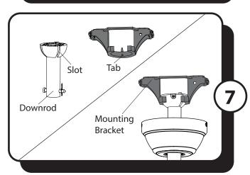
7. Install the ball end of the downrod into the opening of the mounting bracket. Rotate the downrod until the tab in the mounting bracket is seated in the slot in the downrod ball.
