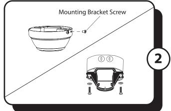
2. Remove the mounting bracket by removing the two mounting bracket screws from the round holes in the canopy. Then loosen the other two mounting bracket screws from the J-shaped slots. Retain the mounting bracket screws for later. Install the mounting bracket to the outlet box (not included) using the screws and washers provided with the outlet box.
