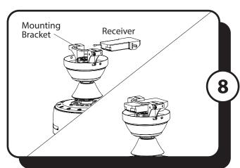
8. Insert the receiver, antenna first, into the mounting bracket with the flat side facing the ceiling.
