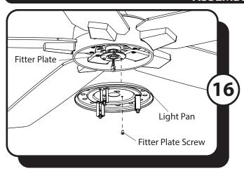
16. Remove one of the three fitter plate screws preassembled to the fitter plate and loosen the other two but do not remove. Feed the 9-pin connector through center hole in light pan. Align the slotted holes in the light pan with the loosened screws in the fitter plate. Turn light pan clockwise and replace the previously removed fitter plate screw. Tighten all screws.
