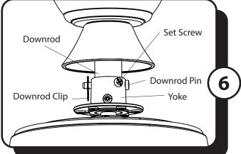
6. Slide the downrod into the yoke of the motor assembly, align the holes, then re-install the downrod pin and downrod clip. Secure with the two set screws and slide the yoke cover down until it rests on top of the motor assembly.
