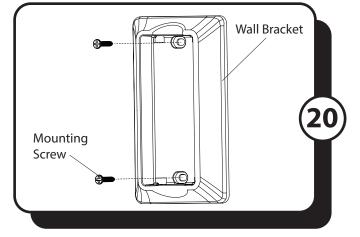
20. If desired, the wall bracket can be installed to the wall using the two mounting screws. Store the remote in the wall bracket when not in use.
