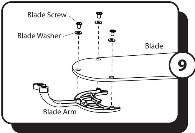
9. Partially insert the blade screws along with the blade washers through the blade and into the blade arm. Tighten each blade screw with a Phillips screwdriver (not included), starting with the one in the middle. Repeat this step for the remaining blades and blade arms.
