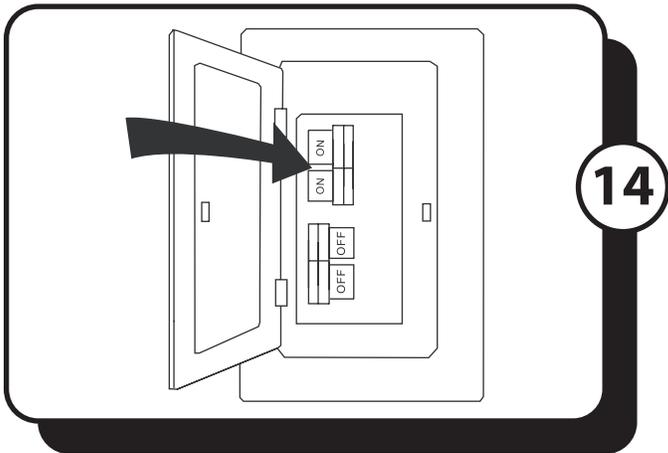
14. Turn on the electrical power at the main fuse or circuit breaker and the wall switch.
