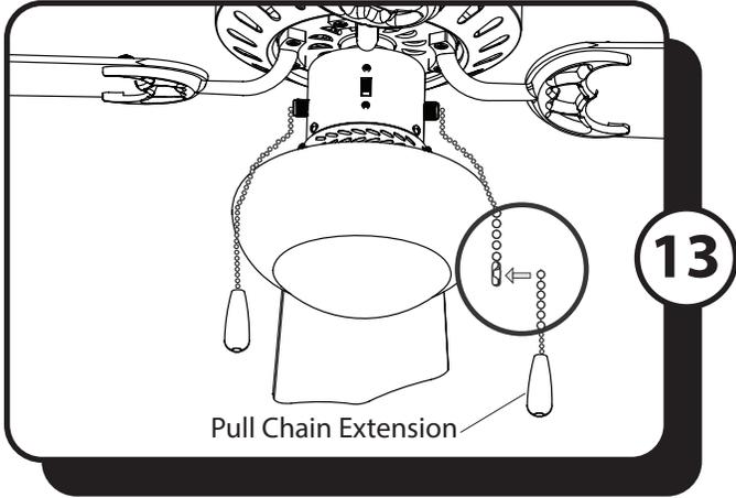
13. Attach pull chain extensions to the pull chains.
