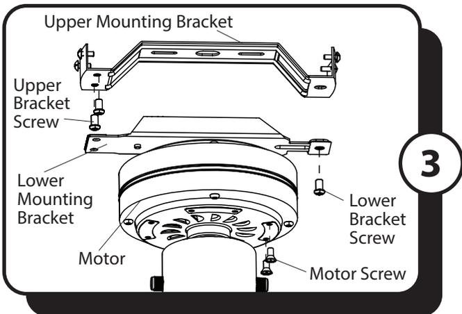
3. Remove the preassembled lower bracket screw from the lower mounting bracket and the upper bracket screws from the upper mounting bracket. Remove the motor screws preassembled to the underside of the motor and set aside for later.
