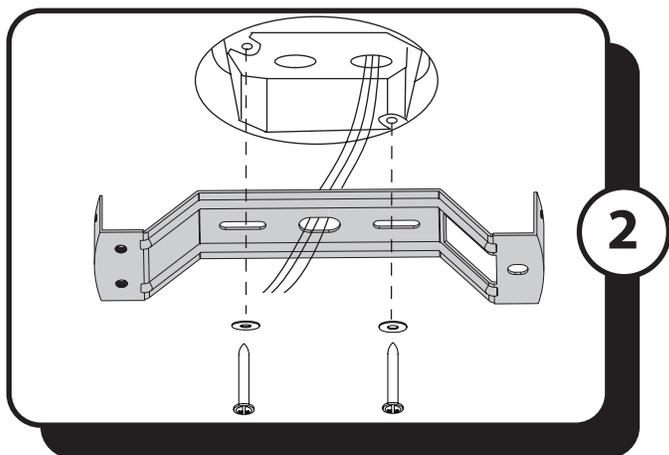
2. Secure the upper mounting bracket to the outlet box (not included) with the screws and washers provided with the outlet box
