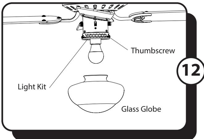
12. Loosen the three thumbscrews near the bottom edge of the light kit. Lift the glass bowl into the light kit and retighten the previously loosened thumbscrews to secure.
