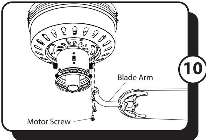
10. Install the blade arm to the underside of the motor assembly with motor screws previously removed (Step 3, page 6). Tighten with Phillips screwdriver. Repeat for each blade arm.
