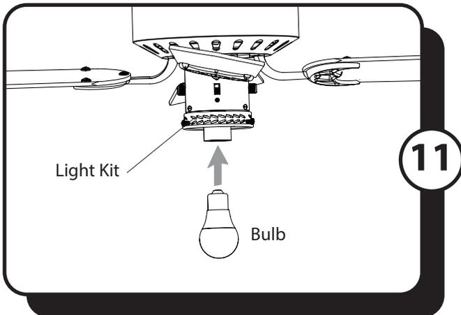
11. Install the E26-base LED bulb into the socket of the light kit.
