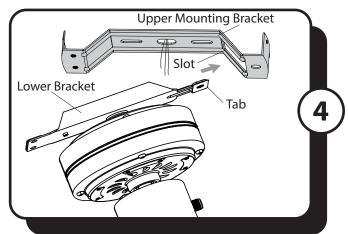
4. Place one tab of the lower bracket into a large slot in the upper mounting bracket.
