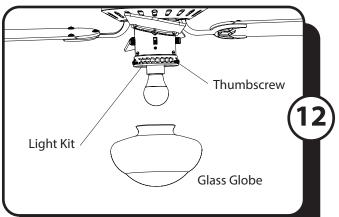
12. Loosen the three thumbscrews near the bottom edge of the light kit. Lift the glass bowl into the light kit and retighten the previously loosened thumbscrews to secure.
