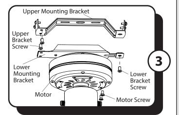
3. Remove the preassembled lower bracket screw from the lower mounting bracket and the upper bracket screws from the upper mounting bracket. Remove the motor screws preassembled to the underside of the motor and set aside for later.
