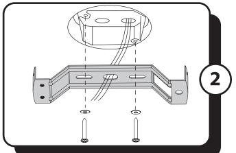
2. Secure the upper mounting bracket to the outlet box (not included) with the screws and washers provided with the outlet box
