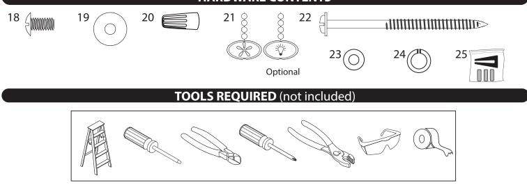
**Tools required for assembly:** Electrical tape, Phillips Screwdriver, Pliers, Safety Glasses, Step Ladder, Wire Cutters and Wire Strippers
