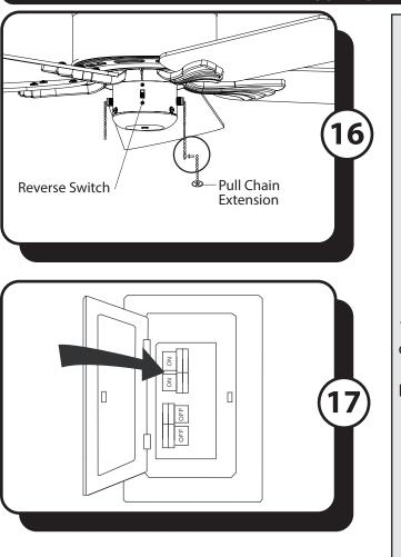
16. Attach pull chain extensions to the pull chains.
