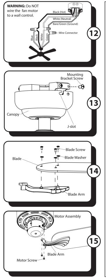
12. Use wire connectors to connect the fan wires to the power supply wires according to the wiring diagram and the following instructions:
