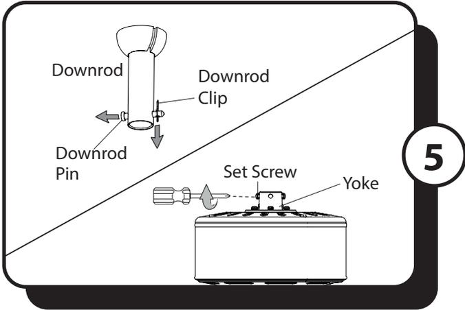
5. **DOWNROD MOUNT** - Remove the downrod clip and downrod pin from the downrod. Then, loosen but do not remove the two set screws at the top of the yoke.
