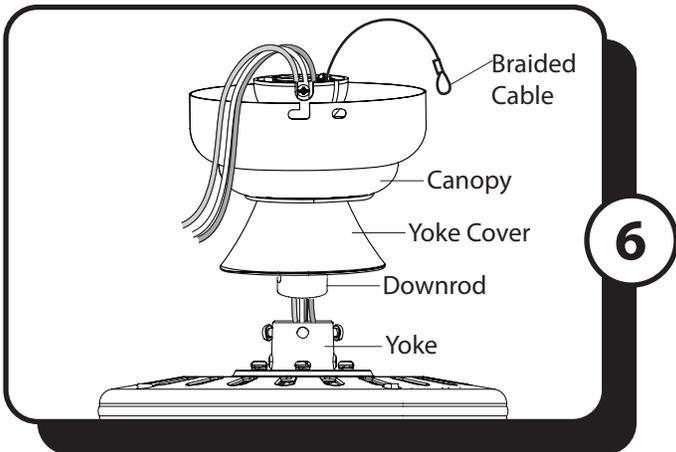
6. Feed the wires and braided cable coming from the yoke through the yoke cover, canopy and downrod.
