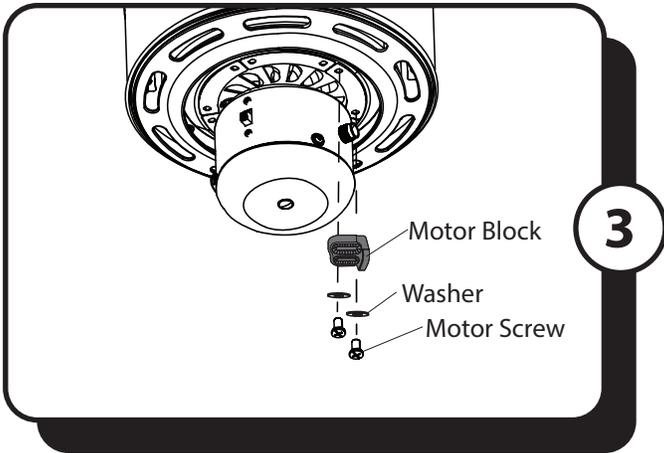
3. Remove the ten motor screws, washers, and five motor blocks from the underside of the motor. Discard the motor blocks but save the motor screws for blade arm installation.
