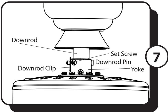
7. Insert the downrod into the yoke and reinstall the downrod pin and downrod clip. Then retighten the two set screws.
