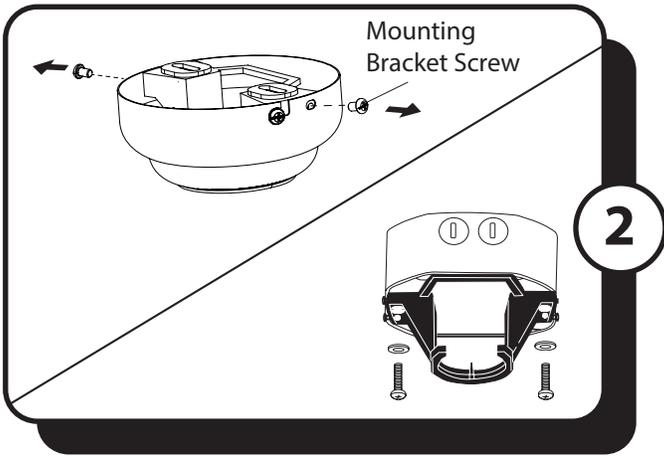
2. Remove the mounting bracket by removing the two mounting bracket screws from the round holes in the canopy. Then loosen the other two mounting bracket screws from the J-slots. Retain the mounting bracket screws for later. Install the mounting bracket to the outlet box (not included) using the screws and washers provided with the outlet box.
