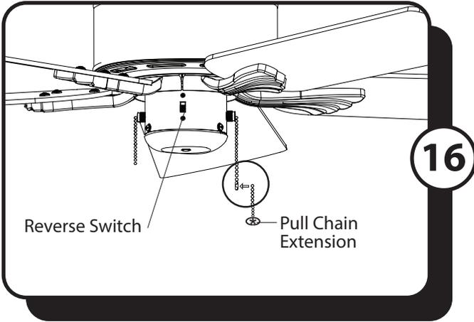
16. Attach pull chain extensions to the pull chains.
