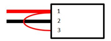
Connect the RED wire (1) to an Ignition-live/positive feed.
